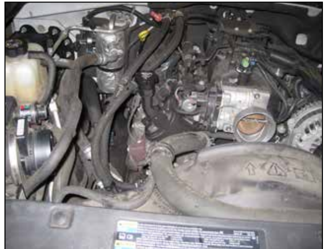
j. Remove the intake duct from the vehicle.
