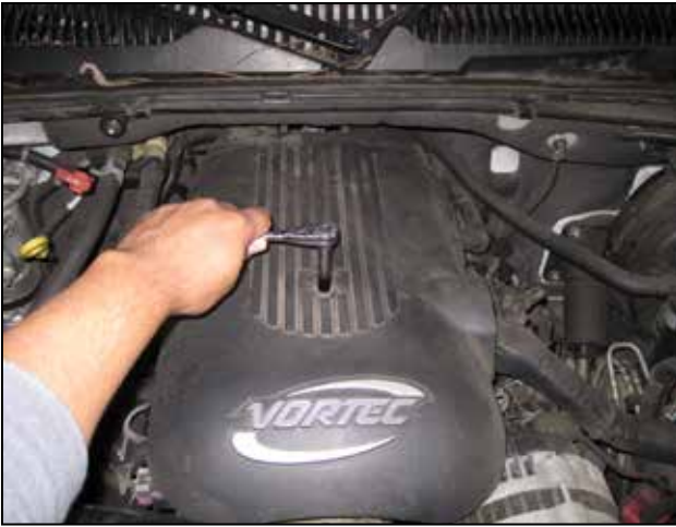
e. Remove the bolt securing the engine cover.
