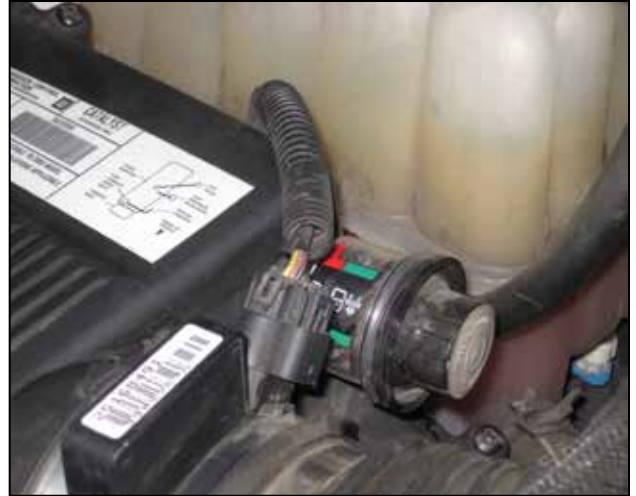
b. Disconnect the mass airflow (MAF) sensor harness.
