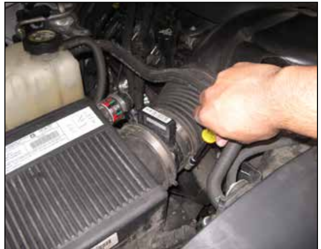
d. Loosen the hose clamp securing the intake duct to the MAF sensor.
