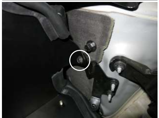
h. Install and tighten the provided bolt from the heat shield to the bracket on the inner fender.
