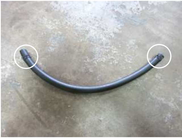
j. Install the spring clamps that were removed in step 2c. onto the provided vent line as shown.
