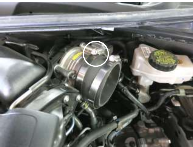
e. Install the provided coupler and hose clamps onto the throttle body. Tighten the hose clamp closest to the throttle body at this time to 30 in. lbs.
