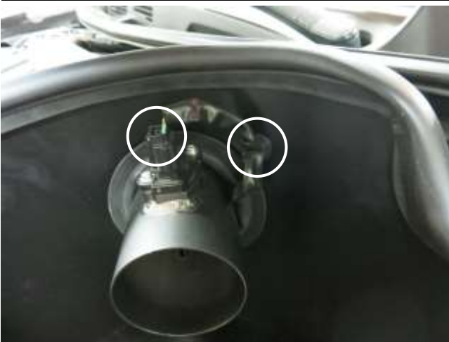
g. Route the MAS harness through the hole via the opening in the bottom portion of the hole, then clip it onto the heat shield and reconnect it back onto the MAS.
