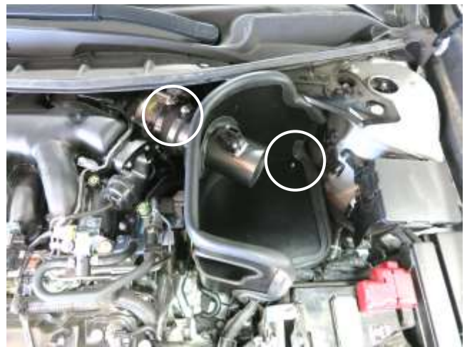
f. Install the heat shield into the vehicle aligning the push in mounts with the vehicles rubber grommets. Then align the AEM intake tube with the coupler.
