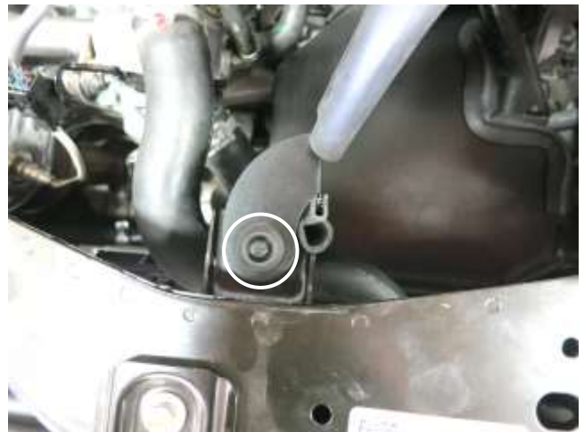
h. Seat the grommet onto the air box post as shown.
