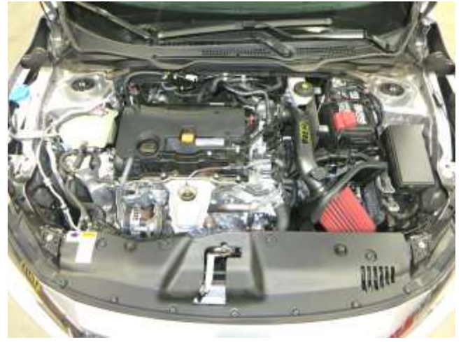
AEM INTAKE INSTALLED
