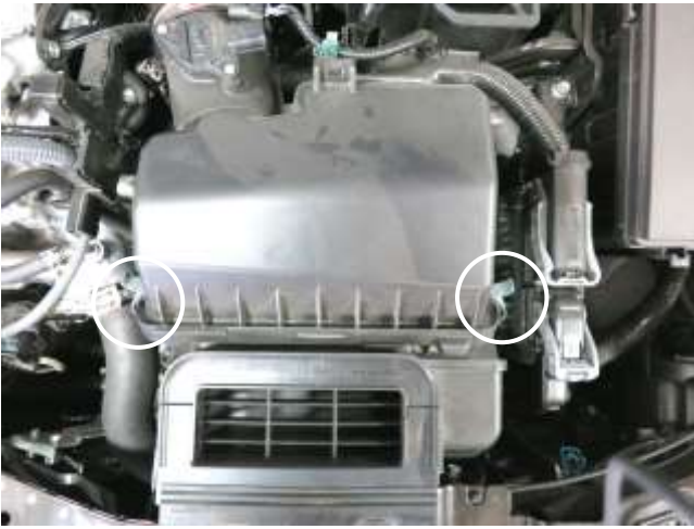
e. Unlatch the two clips on the stock air box.
