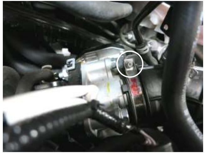
f. Loosen the hose clamp at the throttle body.
