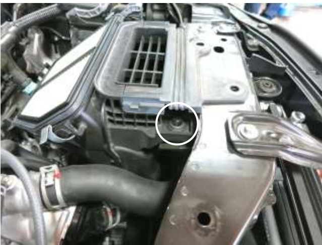
i. Lift the lower air box out of the vehicle making sure to disconnect the grommet from the vehicle.
