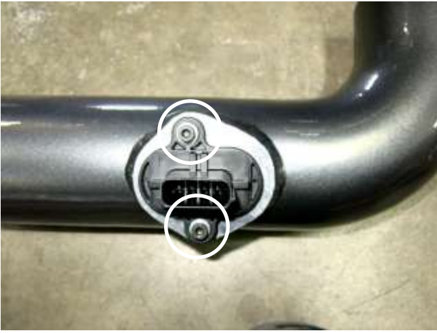
g. Install the mass air flow sensor into the AEM intake tube that was removed in step 2f. and secure with the provided hardware.
