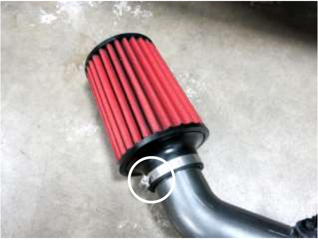
h. Install the AEM filter onto the AEM intake tube and secure with the provided hose clamp.
