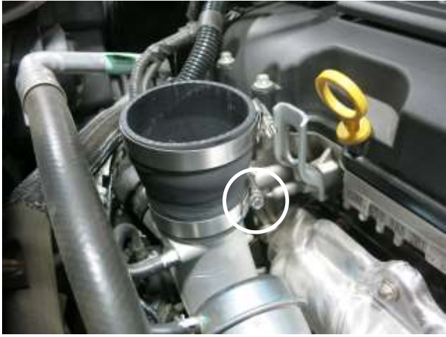
f. Install the coupler and provided hose clamps on to the turbo compressor inlet. Tighten the hose clamp closest to the compressor at this time.
