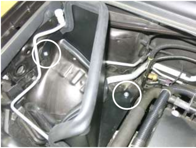
d. Install the completed AEM heat shield into the vehicle aligning the mount on the inner fender and rear rubber grommet.
