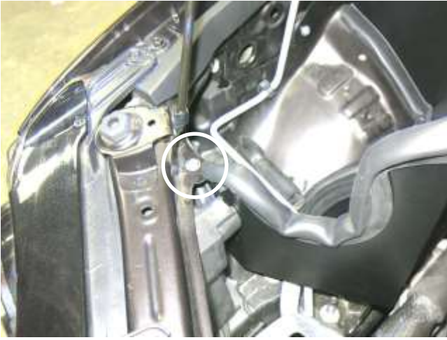
e. Make sure the AEM heat shield is under the lip of the core support, and install the provided bolt/nylon washer securing the AEM heat shield to the vehicle.
