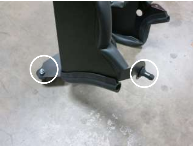
c. Install the provided hardware onto the AEM heat shield as shown. See the diagram on page 2 for parts and part number references.
