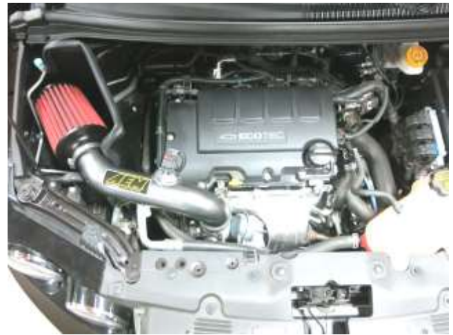
AEM INTAKE INSTALLED
