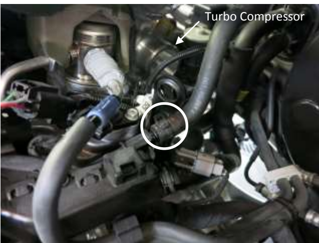
i. Squeeze and work the spring clamp back on the EVAP vent line and remove it from the hard line. Note: You can see the turbo compressor in the back of the picture for reference to locate the vent line.
