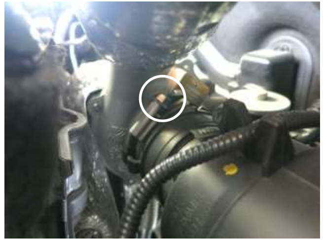
f. Loosen the hose clamp at the turbo compressor.
