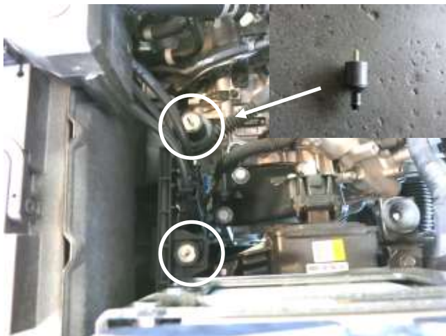
a. Install the provided rubber bushings and plastic mount into the vehicle. Note: You will screw one bushing into the plastic mount as shown in corner of picture.
