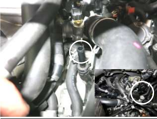
i. Route the previous hose above the “hard line” and too the “T” fitting. Connect the other end of the hose to the “T” fitting and secure with the spring clamp from step 2i. Then, with the two provided vacuum caps, cap the ends of the hard line.
