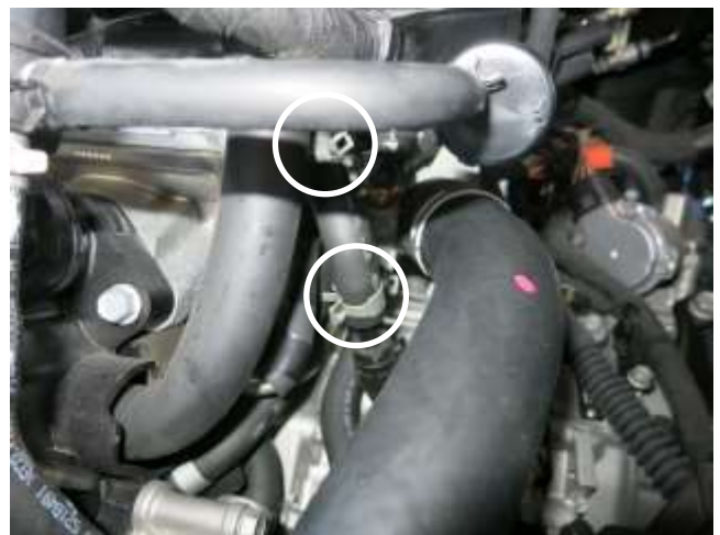
j. Follow the hard line from the previous step to the "T" fitting. Remove the short vent line and spring clamps from the hard line to the "T" fitting. The spring clamps will be reused in step 3f & 3i.
