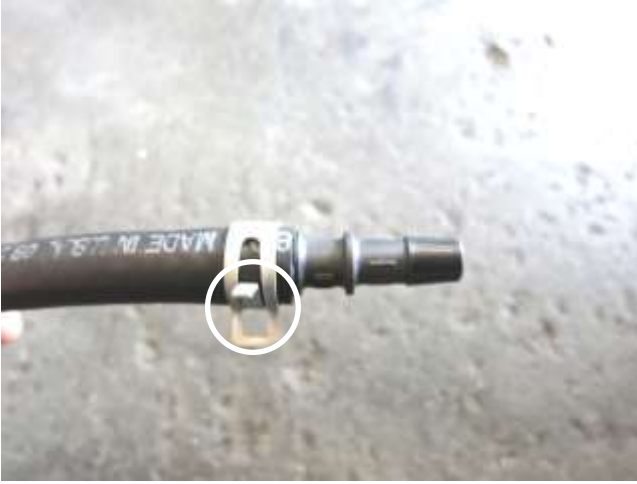
g. Using the providing hose, install the union into one end and secure with a spring clamp removed in step 2j.
