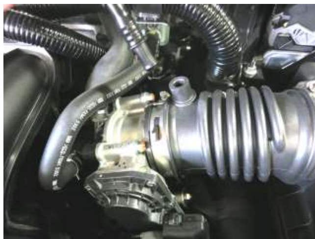
b. Remove breather hose from factory coupler.
