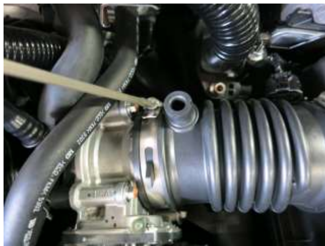
d. Loosen hose clamp securing coupler to throttle body.
