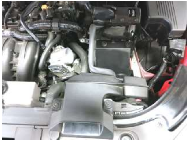
f. Install the AEM heat shield assembly into the engine compartment by lining up the three rubber grommets and secure with factory M6 bolts.
