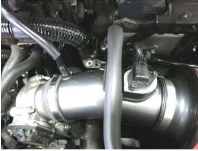
l. Install the breather hose into the coupler and reconnect the MAF sensor wiring.
