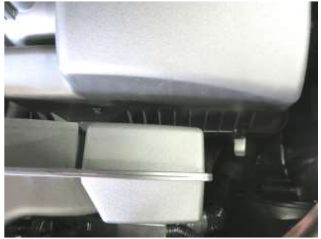
f. Unclip air box lid from lower air box.
