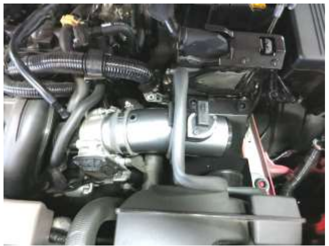
j. Install the AEM intake tube through the heat shield to the throttle body coupler as shown.
