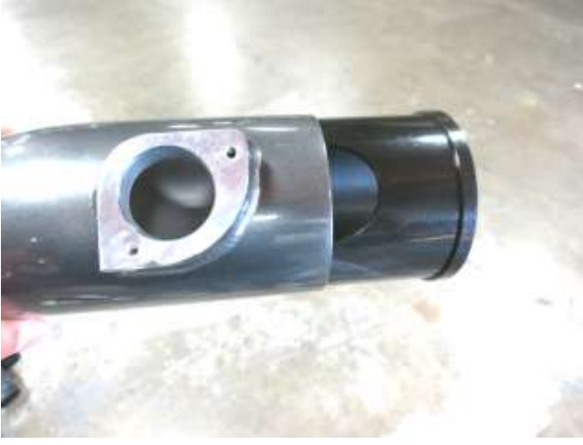
g. Install the supplied MAF sleeve into the AEM intake tube and line up the opening to the MAF adaptor.
