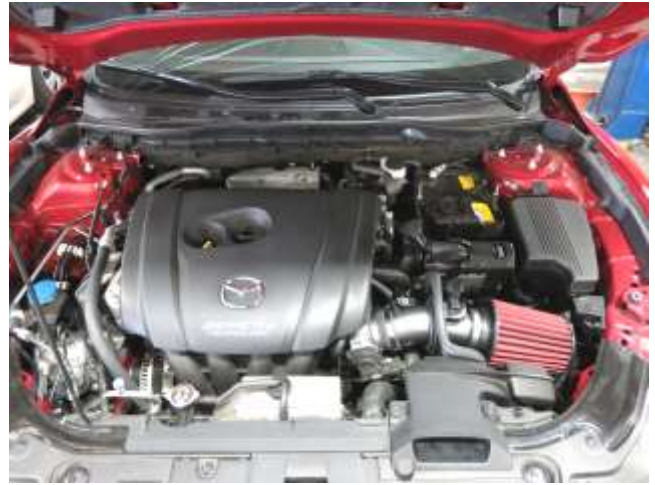
p. Finished installation of AEM Intake System.
