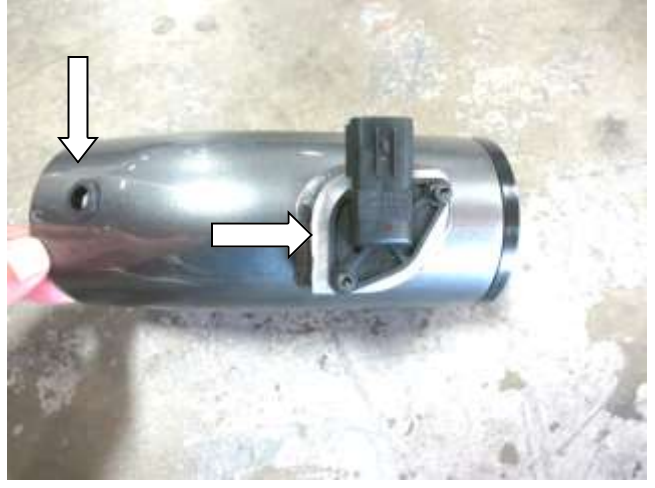
h. Install MAF sensor and rubber grommet into the AEM intake tube as shown.
