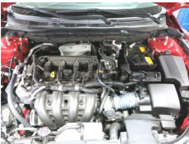
a. Remove engine cover by gently pulling it up and away from the top of the engine.
