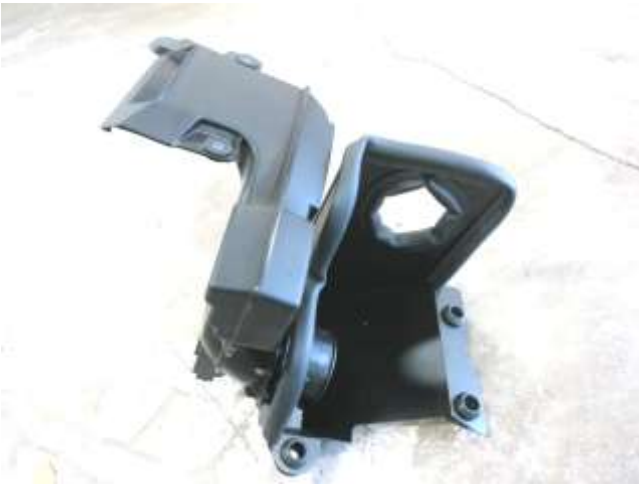
e. Install edge trim around the intake tube pass through hole and around the AEM heat shield then install the air scoop into the AEM heat shield assembly.
