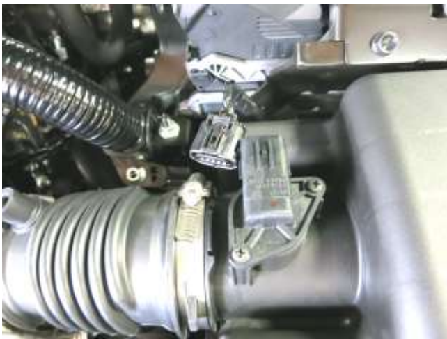
c. Unplug MAF sensor harness.
