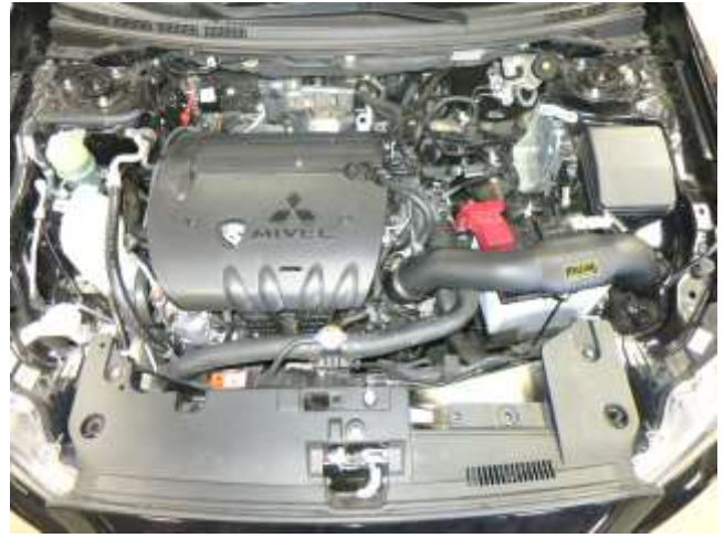
AEM INTAKE INSTALLED
