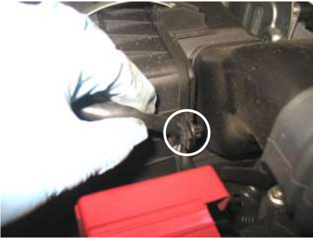
e. Detach the MAF sensor wiring clip from air box.
