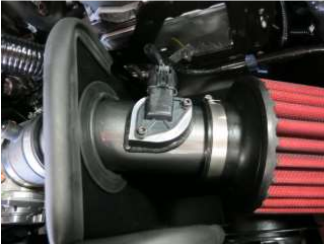
m. Connect the MAF sensor harness to the sensor and tighten all of the hose clamps.
