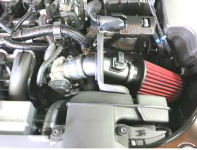
k. Carefully install intake tube and install provided 16" edge trim around top edge of heat shield as shown.
