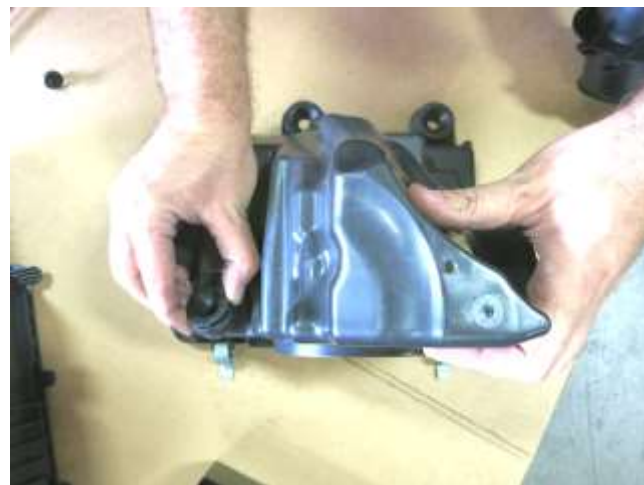
d. Remove the three rubber grommets from the factory air box and insert them into the AEM heat shield.
