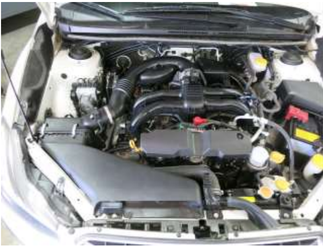
STOCK INTAKE INSTALLED
