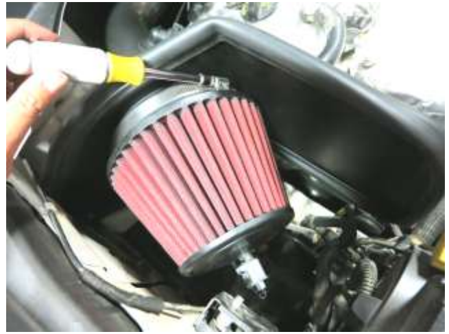
l. Install the air filter and hose clamp(94104) as shown. Connect the IAT harness(21781) to the sensor and check for clearance.
