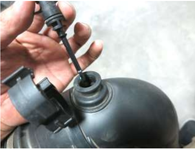
g. Remove the IAT sensor by tilting the lock tab away from the step feature and twist counter-clockwise .
