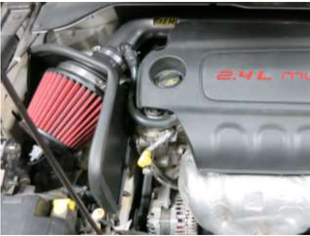
m. Check the harness clearance and snip off excess tabs on zip ties. Reinstall the engine cover and fasten with the stock bolt.
