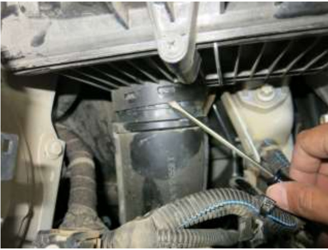
e. Use a flathead screwdriver to detach the inlet duct from the lower air box.
