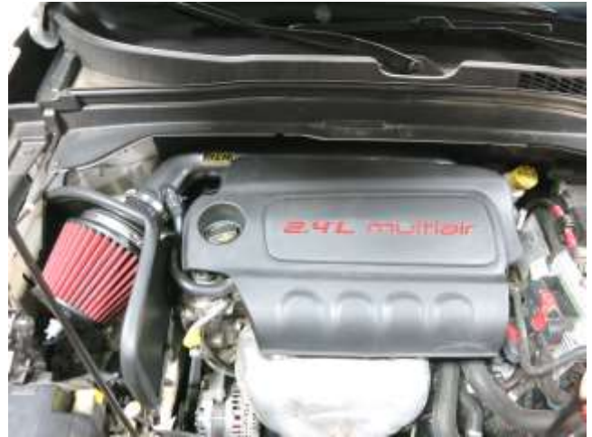
p. Finished installation of AEM Intake System.
