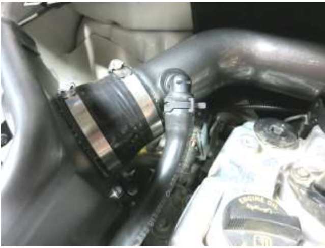
k. Connect the breather hose to the plastic elbow and fasten using the provided spring clamp(08557).
