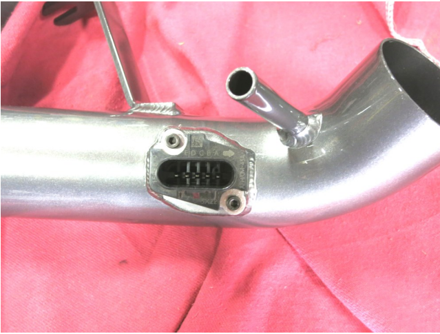
a. Install the Mass Air Flow sensor into the AEM intake tube that was removed in step 2h. with the provided hardware.
