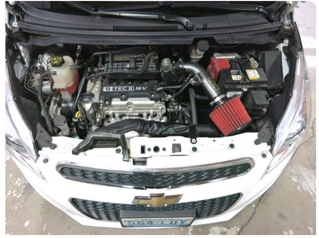
AEM INTAKE INSTALLED
