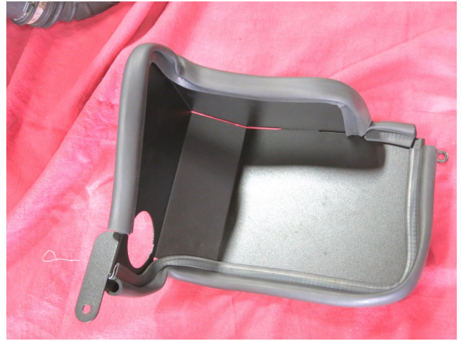
b. Install the provided edge trim onto the heat shield. Trimming of the edge trim may be necessary.
