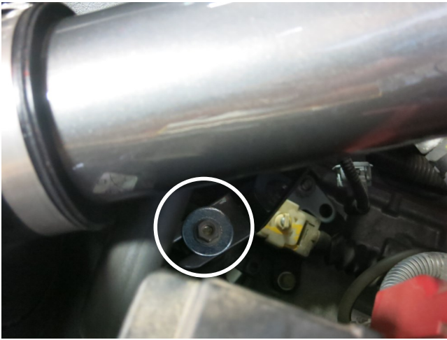
m. Align the AEM intake tube bracket with the stud mount and tighten with the provided washer and nut.
