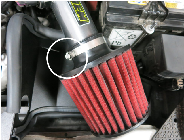
o. Install the AEM air filter onto the AEM intake tube and secure with the provided hose clamp.
