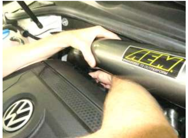
c. Rotate the end of the PCV hose & push it straight in to the corresponding port on the bottom of your new intake tube until fully engaged, then install the tube into the turbo-end coupler. Do not tighten clamps yet.
