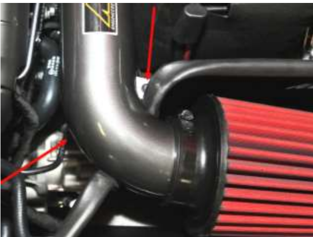
d. Attach the small vacuum hose and install filter. Mount your new intake tube to the rubber mount with the supplied fastener and washer. Do not tighten yet.
