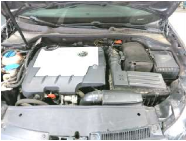
m. Stock intake system
