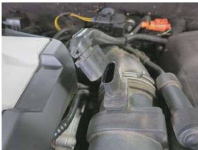
a. Disengage the MAF sensor electrical connector from the MAF sensor.
