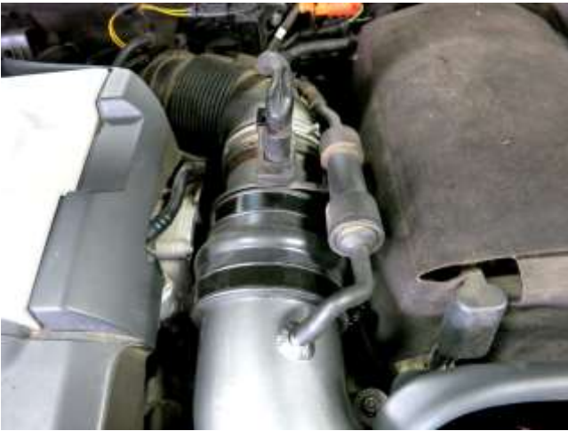
k. Connect the vacuum line to the fitting on the AEM intake tube.
