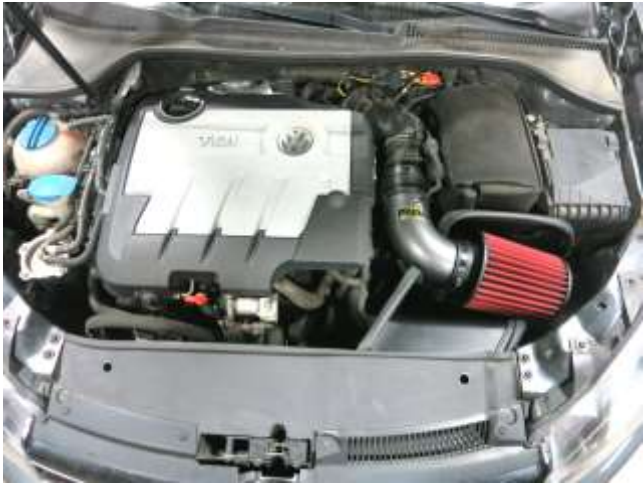
n. AEM air intake system installed
