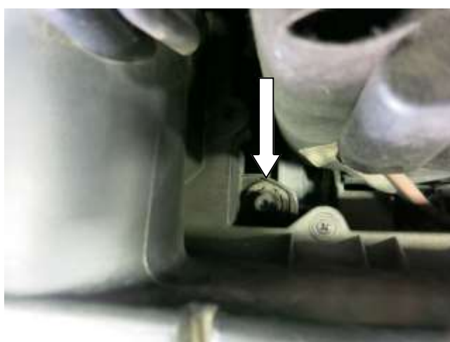
d. Remove the bolt that secures the air box to the air box tray.
