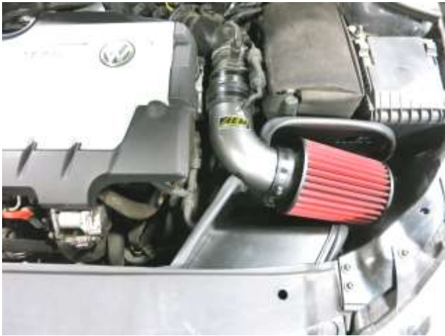
l. When the intake tube is properly aligned, tighten all hose clamps and tighten the M6 nut securing the intake tube bracket.
