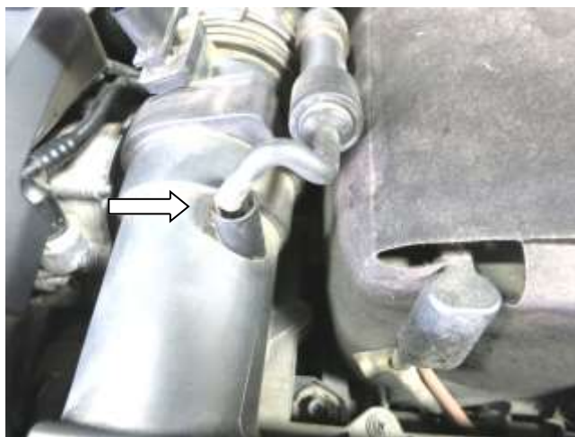
b. Disconnect the vacuum line from the factory air inlet tube.
