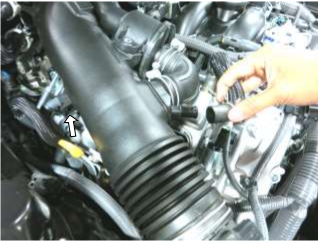
e. Unclip the vacuum hose clip on the lower side of the intake tube. Disconnect the PCV tube as shown.
