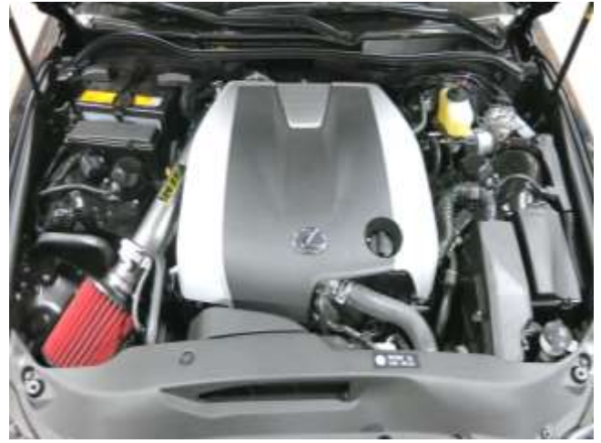
p. Finished installation of AEM Intake System.
