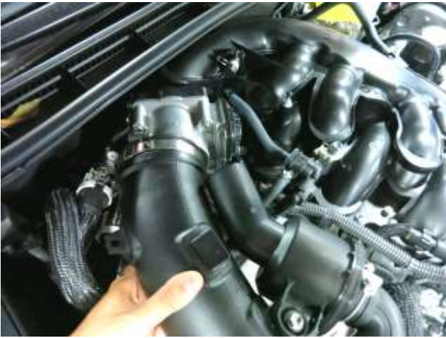
g. Loosen the hose clamp and slide the stock tube off the throttle. Remove the stock intake system.
