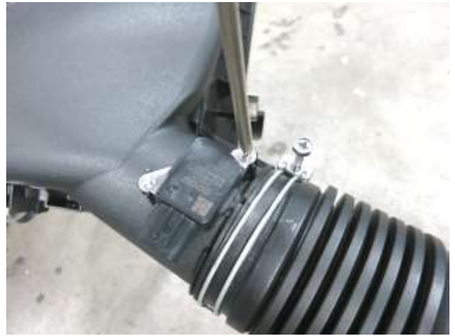
h. Use a Philips screwdriver to remove the MAF sensor from the stock intake tube.
