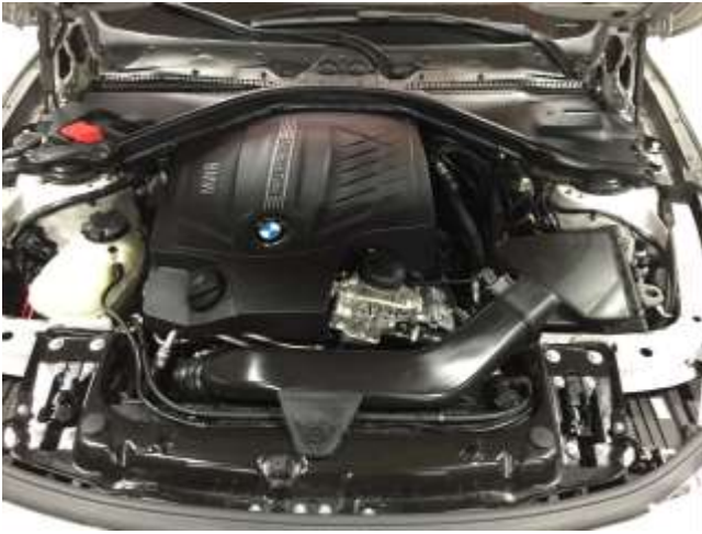
STOCK INTAKE INSTALLED
