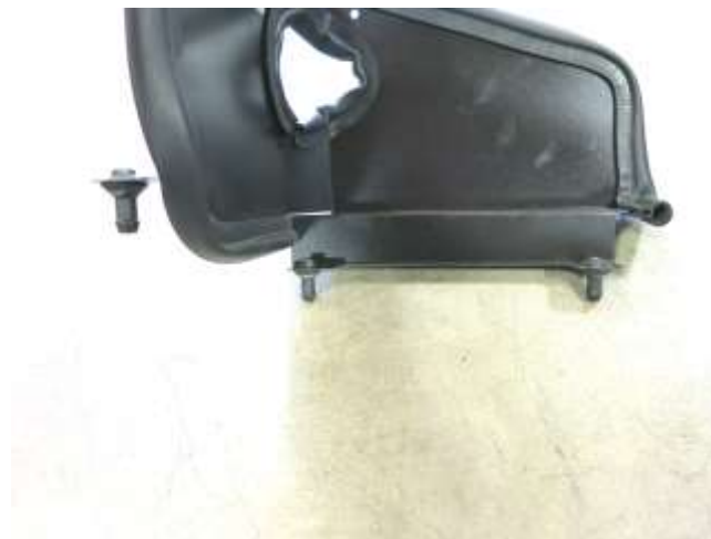
d. Install the bolts and air box mounts to the heat shield as shown.
