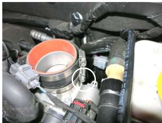
b. Install the coupler with the two supplied (9444) hose clamps and tighten the one closest to the throttle body.
