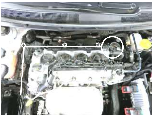
a. Install the extension harness onto the vehicle. Plug one end into the factory connector circled and zip tie the harness to the vehicle where shown.
