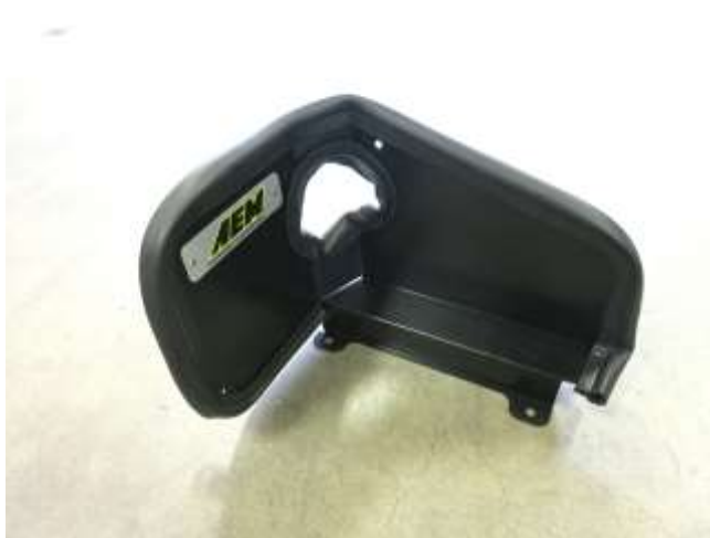
c. Install the two pieces of edge trim onto the heat shield. Note: Some trimming may be necessary.
