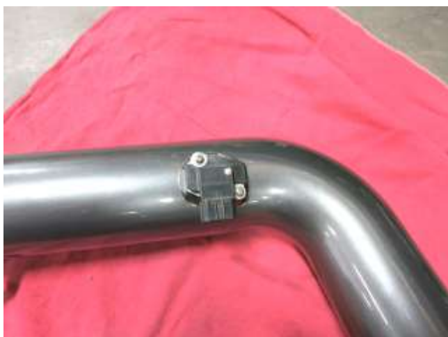
c. Install the MAF sensor and screws into the AEM intake tube from step 2m.
