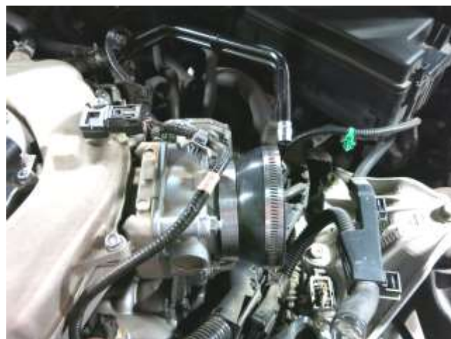
b. Install the included coupler and hose clamps as shown on the throttle body. Tighten the one closest to the throttle body.
