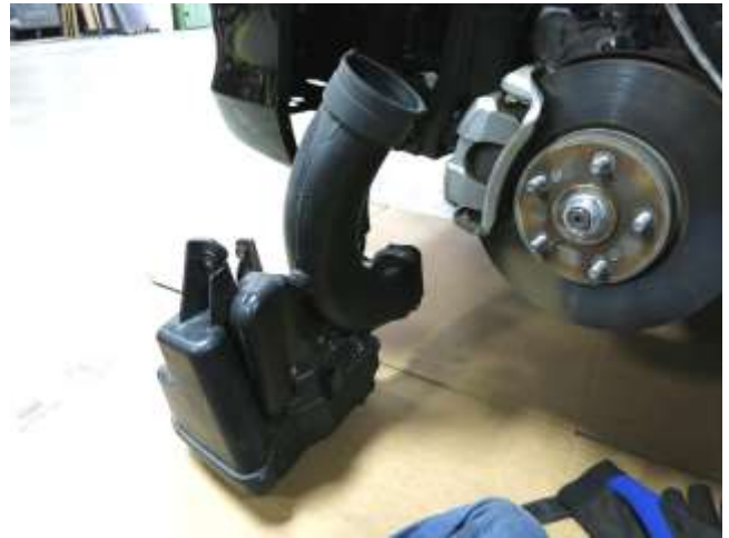
-and remove the bolt on the right. The resonator can then be pulled out as shown above.
