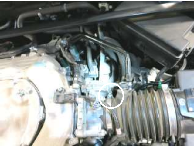
e. Loosen the hose clamp at the throttle body and remove the intake tube from the throttle body.
