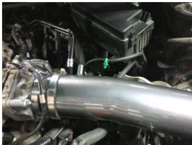
d. Install the AEM intake tube into the coupler that was previously installed. Do not tighten the hose clamp at this time.
