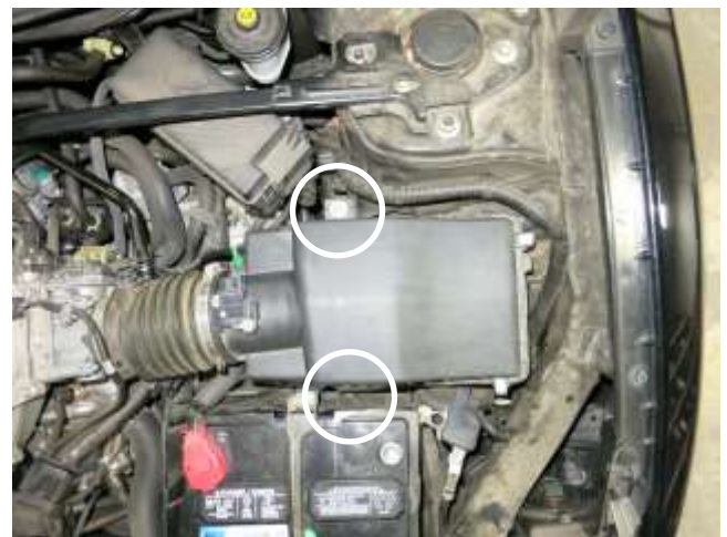
d. Remove the two bolts circled that secure the air box to the vehicle.
