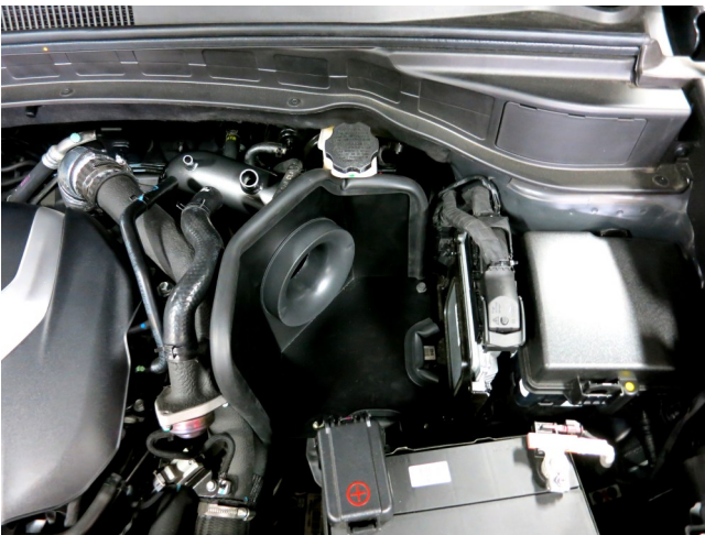
g. Install the assembled heat shield into the vehicle aligning the two slots with the previously installed rubber mounts. Push down to secure the stand-off.
