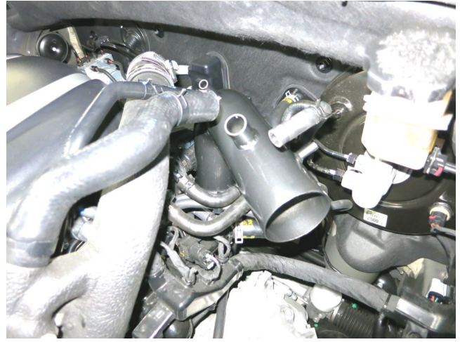
f. Install the AEM intake tube onto the turbo compressor housing. Do not tighten either hose clamp at this time.
