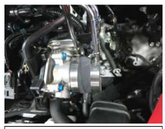
b. Install the transition coupler(08476) and fasten the hose clamp(AEM-9440) over the throttle. Slide loose hose clamp(AEM-9436) over the other coupler end.
