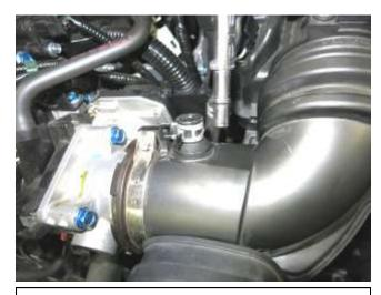
b. Depress the spring clamp on the intake tube to disconnect the hard breather line as shown.
