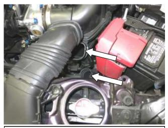
a. Disconnect the upper and lower air inlet ducts from the lower intake box.
