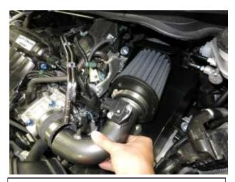
g. Insert the intake tube into the coupler and align the lower rubber mount to the lower bracket.
