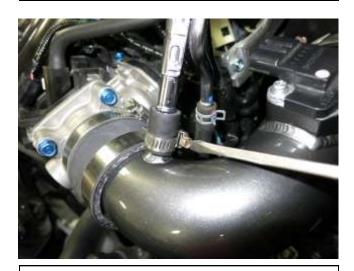
h. Connect the breather line to the intake tube using the hose(AEM-5-1002) and fasten hose clamp(AEM-4093-5). The hose may need top be trimmed for proper fitment.
