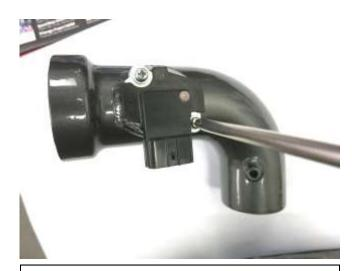
a. Use the stock screws removed in step 2f to fasten the MAF sensor into the AEM tube.
