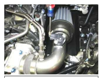
k. Align the filter vertically and tighten the hose clamp to secure its position.
