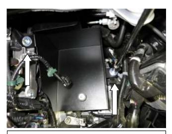
e. Install the heat shield and align locating tabs over the rubber mounts. Fasten tabs down with the provided nuts(AEM-444.460.04) and washers(08160).
