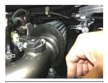
i. Fasten the lower bracket down using the nut(AEM-444.06.04) and washer(08160) provided.
