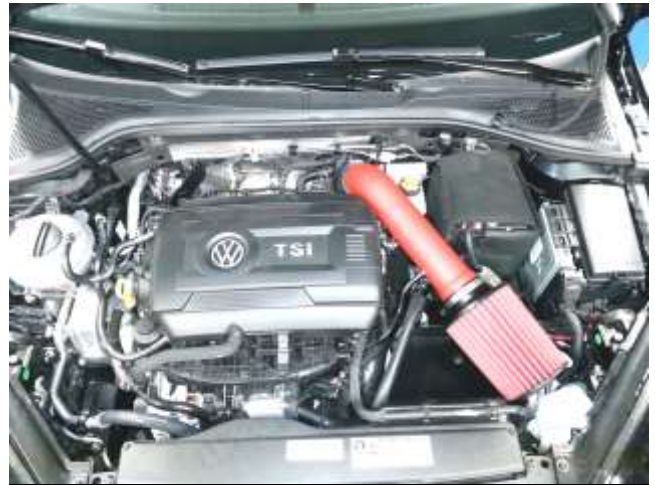
AEM INTAKE INSTALLED
