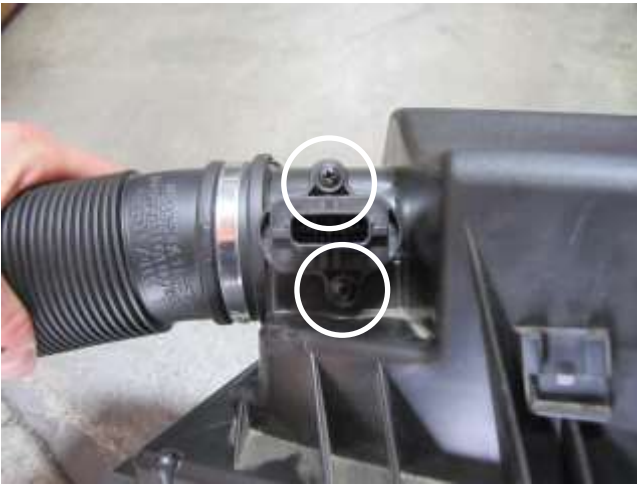
e. Remove the two screws securing the mass air sensor to the air box. Note: The screws will not be reused. The sensor will be reused in step 3h.
