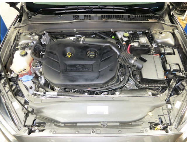
STOCK INTAKE INSTALLED
