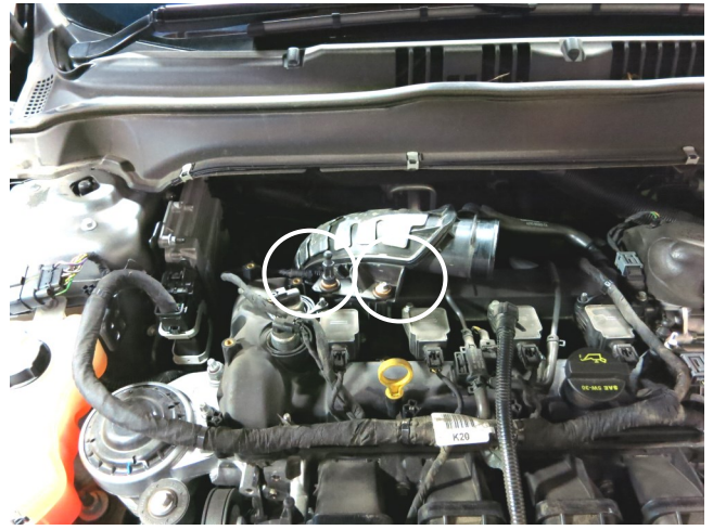
f. Remove the two bolts securing the upper portion of the air intake
