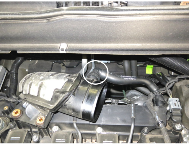
g. Squeeze the connector and slide the connector off of the intake tube.
