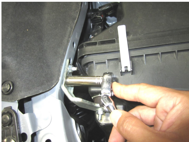
c. Remove the two nuts on the fender that secure the bracket for the air box.
