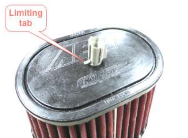
j. Install the IAT sensor into the hole in the end of the filter to the depth of the limiting tab.
