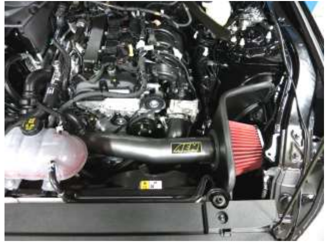
Finished installation of AEM Intake System.
