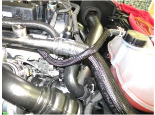
f. Reinstall the PCV hose by pushing it down over the quick disconnect fitting until it clicks.
