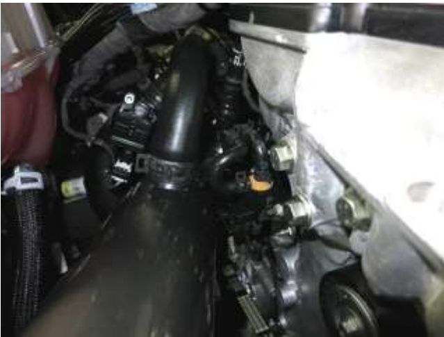
g. Reinstall the recirculation hose over it's corresponding tube port and engage the spring clamp.
