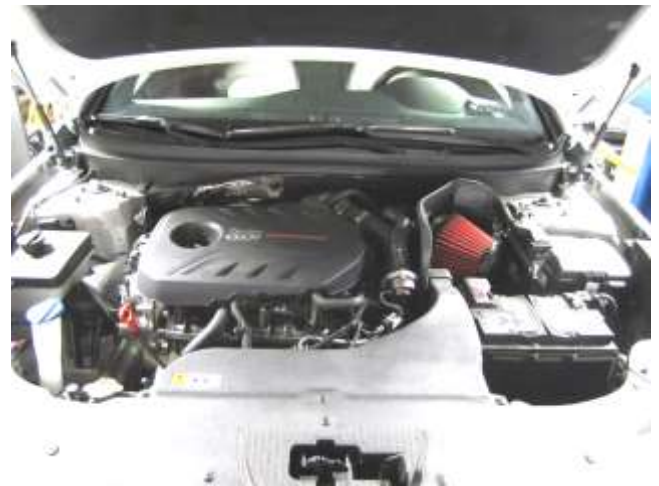
AEM Intake Installed
