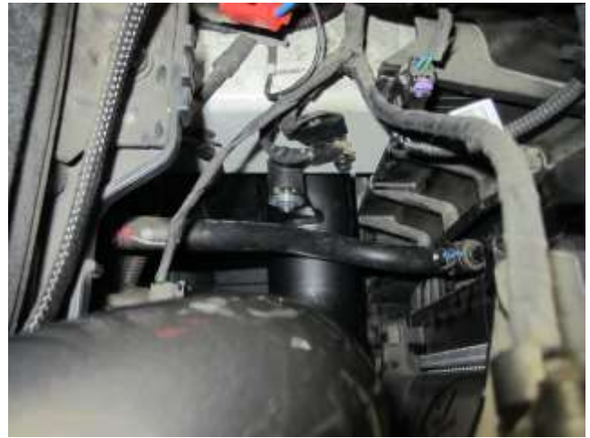
d. Slide the tube into the wheel well, align the bracket with the rubber mounted stud. Install/tighten the washer and nut to secure the tube. Note: The tube will go between the two flex lines that run to the radiator.
