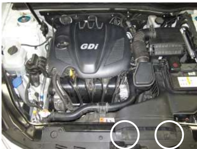
a. Remove the engine cover by pulling up and out of the vehicle. Remove the two bolts holding the air scoop to the vehicle and remove the scoop.
