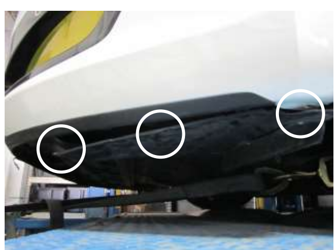
h. Remove the 3 screws holding the drivers side splash guard and lower the guard.
