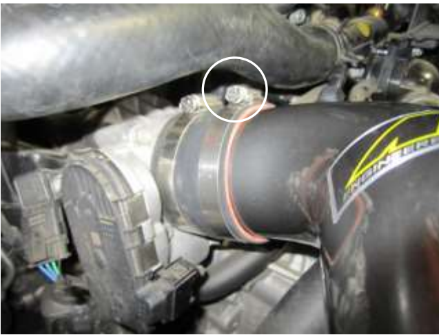
e. Install the tube into the throttle body coupler and tighten the hose clamp. Note: Make sure there is clearance between tube and coolant lines.
