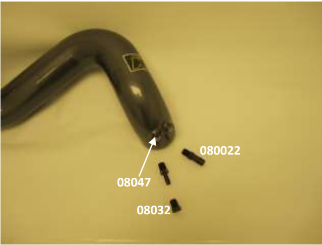
c. Install the correct fitting based on your vehicle vent line configuration. On vehicles equipped with an EVAP vent line use the fitting (08047). On vehicles not equipped, use the plug (08032).
