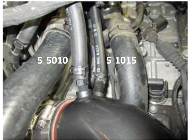
f. Install the hose (5-5010) and (5-1015) onto the fittings and secure with the pressure clamps that were removed in step 2d.
