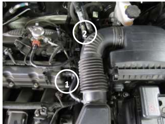
d. Loosen the #1 pressure clamp and remove the vent tube. On vehicles equipped with an EVAP vent line, disconnect the #2 pressure clamp and remove the EVAP hose from the "T" fitting. All four of the pressure clamps will be re-used in 3f & 3g.
