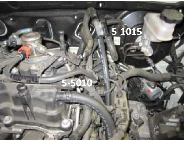
g. Install the other end of hose (5-5010) onto the valve cover port. Install (5-1015) onto the EVAP vent line. Secure with the pressure clamps removed in step 2d.
