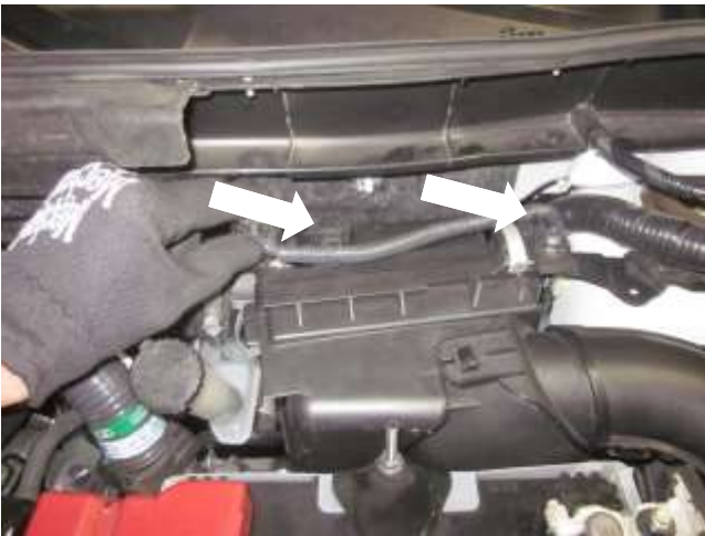
a. Unplug the MAF sensor connector and disconnect the two clips holding the wiring harness to the airbox.
