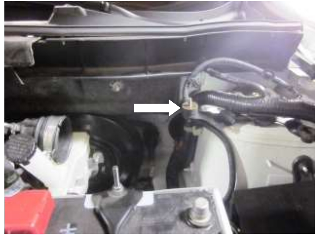
b. Install one of the provided rubber bushings in the bracket where you removed the M6 bolt in step "C" and tighten.
