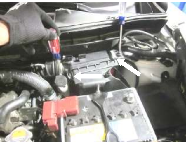
c. Loosen the hose clamp, remove the M6 bolt, and disconnect the two latches securing the air box together.
