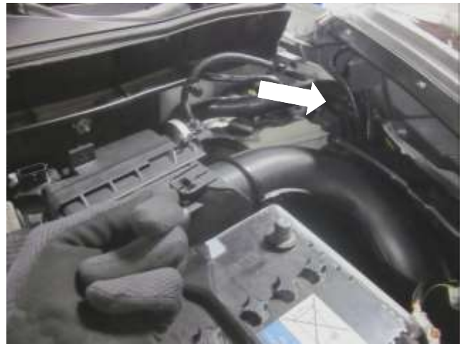
b. Lift up on the air box tab and pull out the locating pin on the stock air intake tube.
