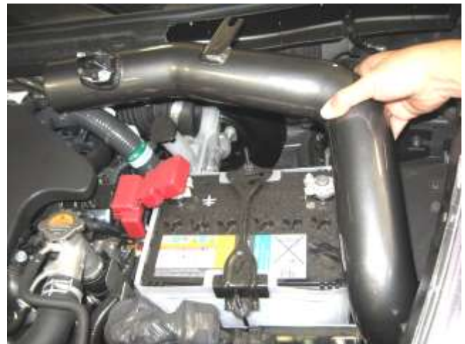
d. Install the AEM intake tube by inserting it into the opening next to the battery and into the lower fender well first, and then gently maneuver it into position.
