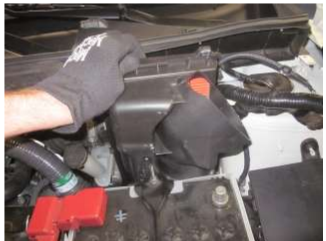
d. Remove the front half of the air box with the filter intact by lifting out of the vehicle.
