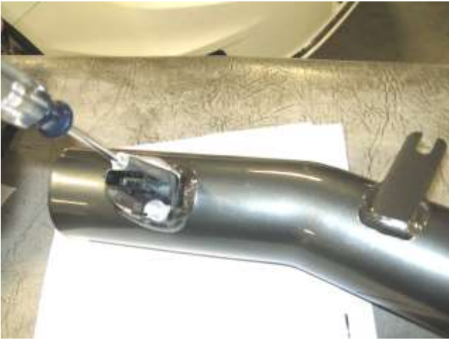
a. Install the MAF sensor and two M2 screws that were removed in 2j and tighten into the AEM intake tube.
