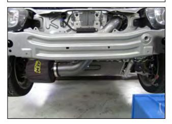
h. Re-install the front bumper assembly using the 8 factory bolts. Ensure the air filter or intake tube does not contact any part of the vehicle.
