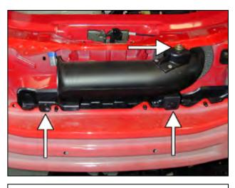
p. Remove the inlet air tube by removing the two retaining clips and the bolt securing it to the chassis.
