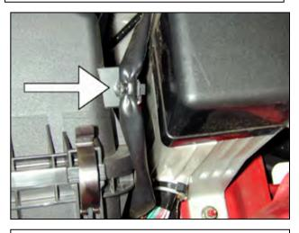
c. Unclip the MAF sensor wiring harness from the side of the air filter housing.
