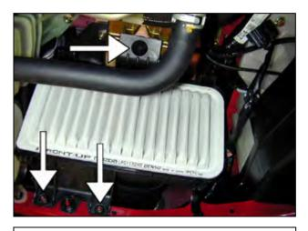
e. Remove the lower air filter housing and filter by removing the two nuts securing the housing to the chassis. Next, lift up on the back side of the housing and remove it from the vehicle.
