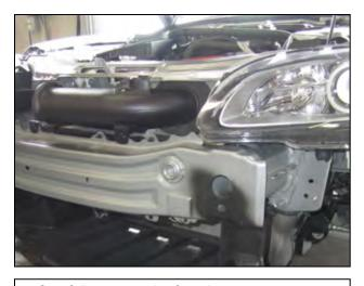
o. Carefully remove the front bumper cover to reveal the stock inlet air tube and the bumper assembly.
