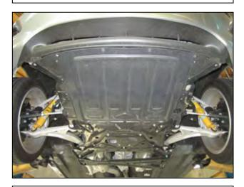
h. Remove the clips and bolts securing the center splash shield to the vehicle. Remove the splash shield.
