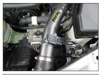
b. Install the AEM® upper intake tube (D) into the stock elbow coupler at the throttle body as shown. Secure using the stock hose clamp. Connect the MAF sensor wiring harness to the MAF sensor.
