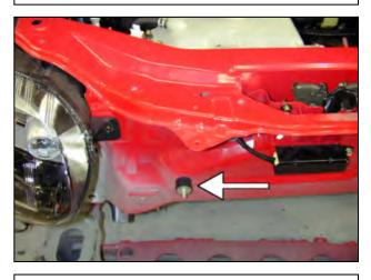
d. Install the other M6 isolator mount (F) in the location shown. Secure using the supplied M6 flat washer (G) and M6 nut (H).
