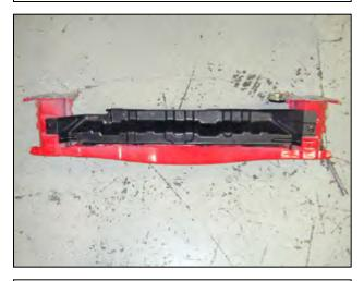
t. Remove the splash shield by removing the plastic clips securing it to the bumper assembly.
