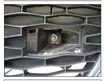
k. Remove the 2 small plastic covers in the grille fascia to reveal 2 bolts securing the bumper cover to the bumper support. Remove the 2 bolts.
