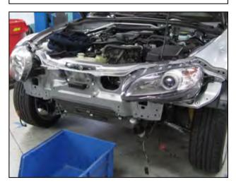
s. Remove the 8 large bolts securing the bumper supports to the chassis. Remove the bumper beam assembly.
