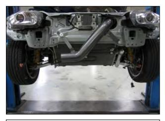
e. Loosely mount the lower intake tube (A) brackets to the isolator mounts as shown using 2 flat washers (G) and 2 M6 nuts (H) turned finger tight.
