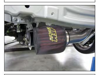
j. Position the AEM® intake for best fitment. Tighten the nuts on the mounting brackets. Re-adjust the pipe if necessary.
