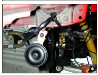
i. Re-install the clip for the horn wiring harness from the horn to the front bumper support. Re-install the clips attaching the IAT sensor and wiring harness to the bumper beam.
