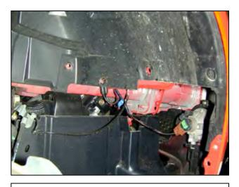
j. Remove the clips and bolts securing the passenger side front fender liner and remove the liner. Disconnect the fog light and side marker light from the wiring harness.
