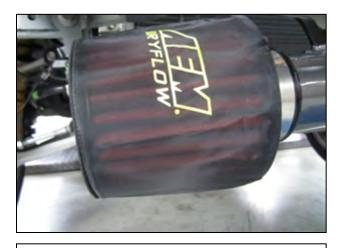
g. Install the AEM® prefilter (L) over your new AEM® Dryflow air filter (B), then mount the filter onto the end of the lower intake pipe using the #52 hose clamp (K) and fully tighten.
