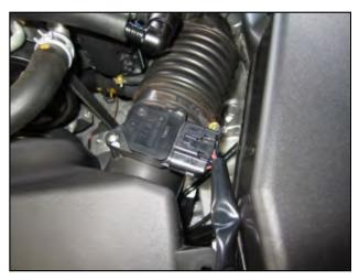
a. Loosen the hose clamp securing the air box outlet tube to the flexible elbow coupler at the throttle body. Disconnect the coupler.
