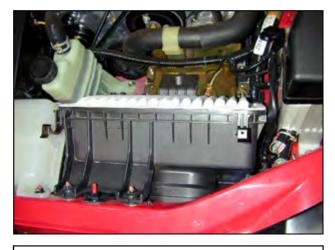
d. Remove the upper air filter housing by unhooking the metal retaining clips and sliding it out.
