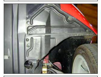
g. Remove the retaining clips and bolts securing the passenger side splash shield to the vehicle. Remove the splash shield.
