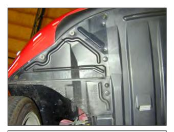
f. Remove the retaining clips and bolts securing the driver side splash shield to the vehicle. Remove the splash shield.
