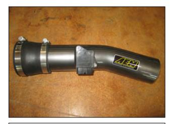
a. Install the MAF sensor into the upper intake tube (D) and secure using the two supplied 8-32 Allen bolts (E). Install the reducing coupler onto the end of the intake pipe and secure with the #44 hose clamp (I). Loosely install the larger #48 hose clamp (J) onto the end of the coupler.
