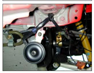
r. Disconnect and unhook the wiring harness from the horn attached to the front bumper support. Unhook the clips attaching the IAT sensor to the bumper beam. Remove the plastic clips securing the plastic splash shield to the bumper support and the chassis.
