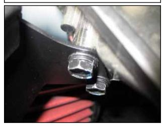
q. Reinstall the OEM M6 bolts in the factory mounting bracket location.
