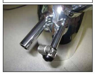
i. For automatic cars use the provided cap (R) and hose clamp (S) to cap off the vent tube.
