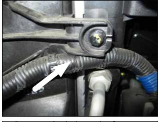
Remove the bolt on the fan shroud.
