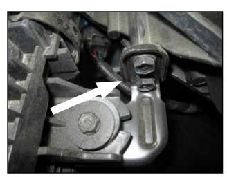
c. Loosen & remove the two M6 bolts securing the air box bracket that secures the air box bracket to the radiator core support.
