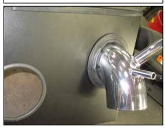
j. Place intake tube (B) through the hole in the heat shield (O) as shown.
