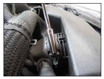
b. Loosen the hose clamp on the intake pipe.
