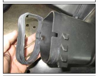
j. Remove the seal from the air box.
