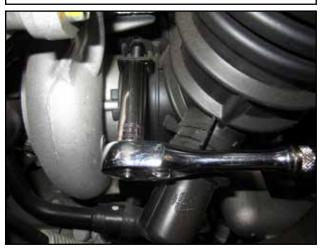
h. Loosen the hose clamp securing the stock tube onto the turbo inlet.
