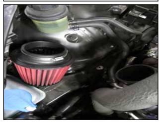
h. Place filter (E) and hose clamp (F) in the engine bay as shown.
