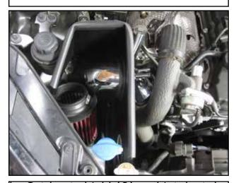
k. Set heat shield (O) and intake tube(B) in place.
