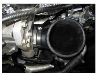
d. Install the coupler (H) onto the Turbo inlet using the provided hose clamps (G) and (I).
