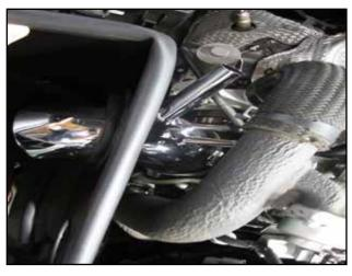
Install intake tube (B) into coupler (H) .
