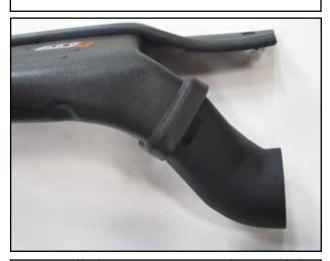
u. Install the AEM scoop adapter (A) into the OEM ducting.
