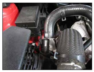
Remove the recirculation hose on the OEM intake pipe.
