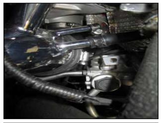
s. Reconnect the PCV hoses and fasten with the OEM spring clamps.
