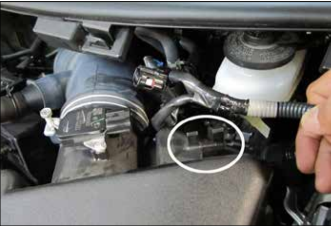
c. Disconnect wire harness from MAF sensor and unclip MAF wire harness from stock airbox.
