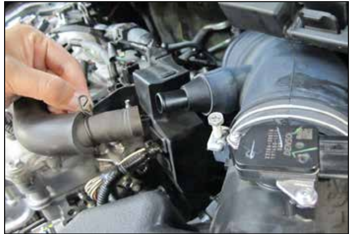
d. Pinch and slide back the black spring clamp on the valve cover hose. Twist valve cover hose to disconnect from intake tube.
