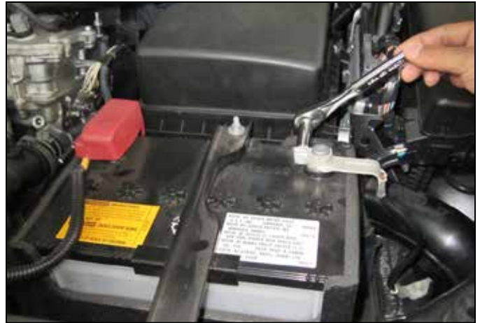
b. Disconnect negative terminal on battery using 10mm socket and tuck away from battery.
