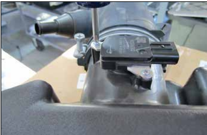
m. Remove the MAF sensor using a Phillips head screwdriver and set aside for later use during the AEM® intake installation.
