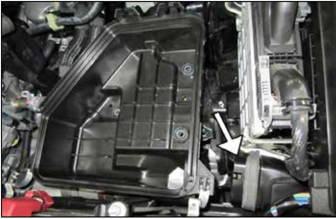
k. Disconnect lower airbox from inlet tube. Remove the lower airbox and set aside.
