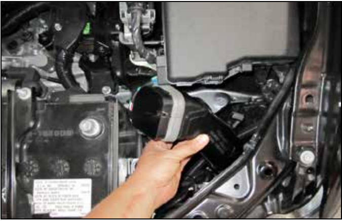
l. Slide the inlet tube down towards the headlight slightly and remove the inlet tube from the vehicle.
