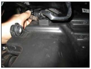
Carefully lower the intake resonator and disconnect the tree mount clip to detach the foglight harness. Set aside resonator chamber.
