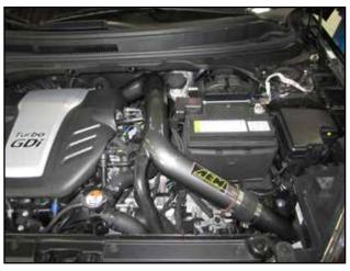
AEM cold air intake system installed.
