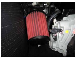
g. Check for clearance around filter between fog light housing and also plastic liner. Adjust the position of the lower tube if necessary. Tighten hex nuts(H) and hose clamps(C) once filter is properly positioned. Reinstall lower belly pan cover and plastic well liner.
