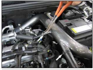
Reconnect crank case breather hose and recirculation valve hose to upper tube(A) and fasten using stock spring clamps as shown.
