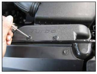
Remove the two plastic clips shown above and pull up on the air inlet snorkel to remove.
