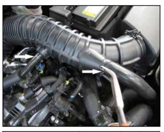
Loosen spring clamps to detach crank case breather hose and recirculating valve hose from intake tube.
