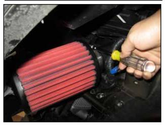
From the driver's side wheel well, install filter(E) onto lower pipe and secure with provided hose clamp(F).
