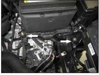
Install the two rubber mounts(I) provided into the previous mounting location of the stock aibox as inidicated.
