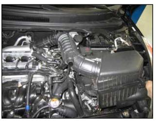
Firmly grasp the airbox and slide it towards the engine to detach from lower chamber. Remove stock intake airbox and tube assembly.
