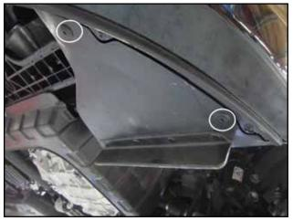
Remove the two plastic clips under vehicle, near driver's side front wheel to lower plastic wheel well liner.
