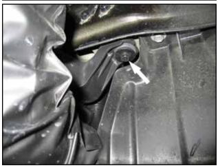
j. From driver's side wheel well, remove the M6 bolt used to secure the intake resonator chamber rear mount.
