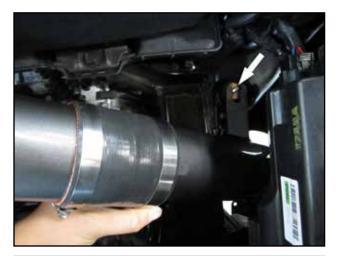
d. Slide provided coupler(B) over non-stamped end of lower pipe(D) along with two hose clamps(C).
