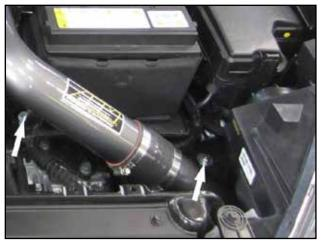
f. Use the provided hex nuts(H) and washers(G) to loosely fasten upper and lower tubes to the rubber mounts previously installed.
