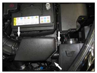
Remove the three M6 bolts securing the stock airbox
