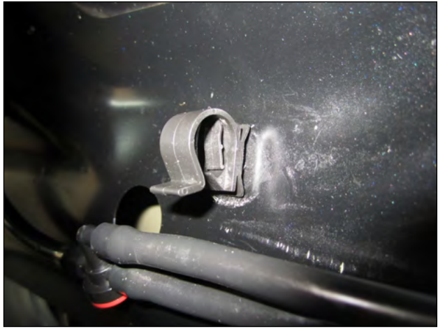
h. In most vehicles, you will need to disengage the washer fluid hose from the middle clip at the rear of the hood. Remove the clip and orient the check valve on the hose as shown.
