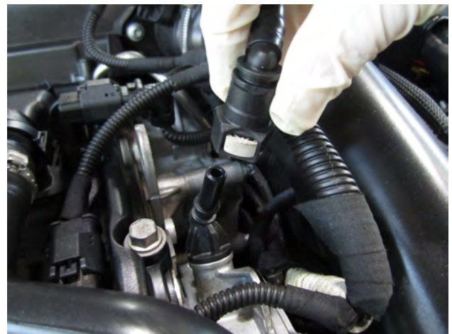
d. Disconnect the vacuum line port.
