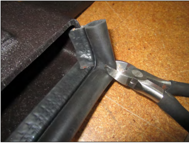
g. Cut reliefs in the 2 bent corners of the bulb seal. This will allow the bulb seal to conform to the shape of the hood.
