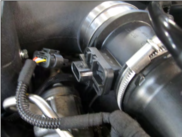
a. Disconnect the harness from the MAF sensor.
