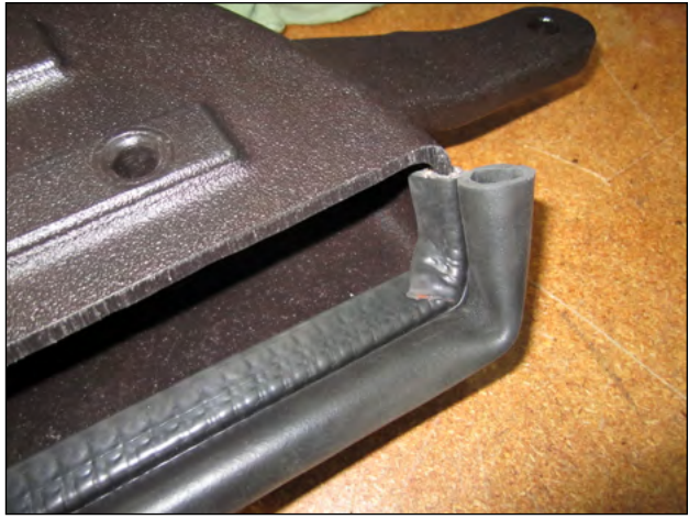
f. Install the edge trim bulb seal onto the lower edge of the AEM® cold air intake scoop. Overlap the slit ends to prevent binding around the 2 lower corners. Fully seat the trim with a rubber mallet or your hand.
