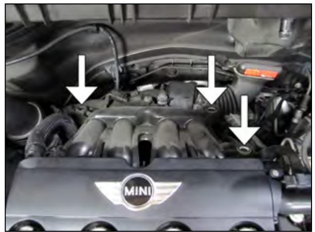
e. Pull up on the stock air box assembly carefully until it pops free from the 3 rubber mounting grommets on the intake manifold. Make sure all 3 rubber grommets stay in the intake manifold.
