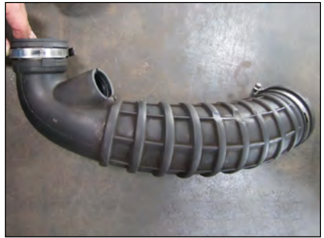
b. Loosen the hose clamp connecting the intake tube to the turbo inlet. Disconnect the PCV hose to completely remove the intake tube.
