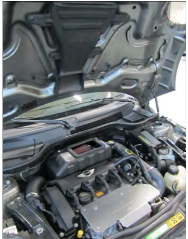
AEM® Cold Air Intake installed
