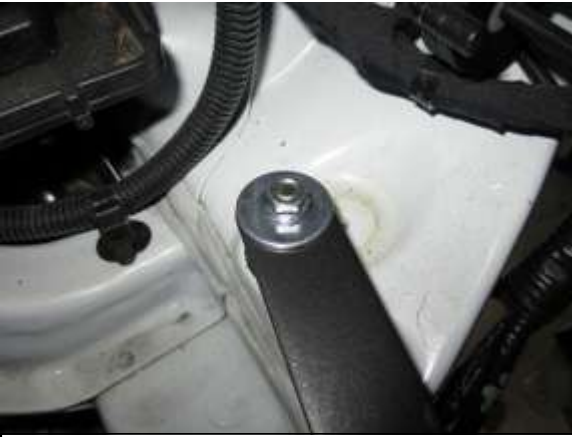
E. Loosely install the flat washer (C) and M6 flanged hex nut (D) over the M6 mounting stud as shown. Do not tighten yet.
