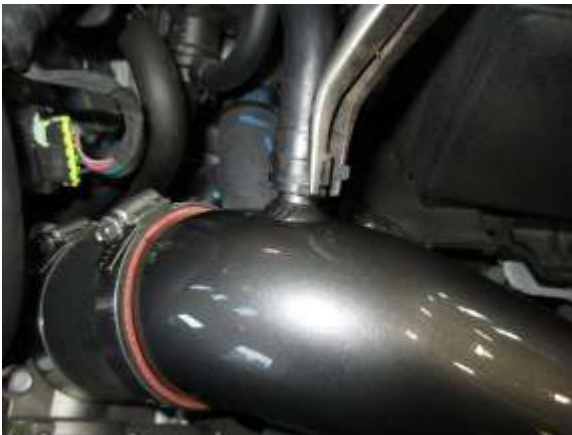
G. Connect the breather hose onto the intake tube at the breather nipple using the stock clamp as shown.
