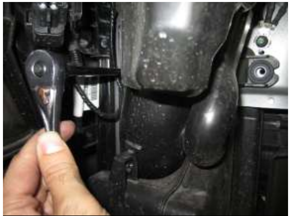
L. Inside the wheel well area, remove the 3 M6 bolts retaining the intake silencer to the frame support.
