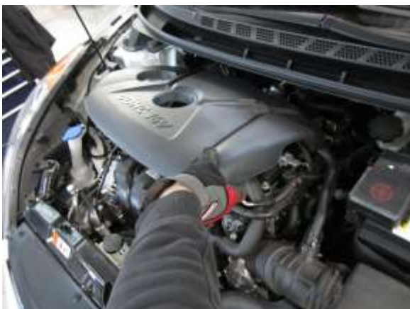
A. Open vehicle hood. Remove the plastic engine cover.
