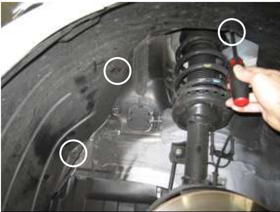
K. Unscrew and remove the 3 front plastic clips retaining the drivers' side fender liner. Pull the fender liner aside to expose the stock intake silencer.
