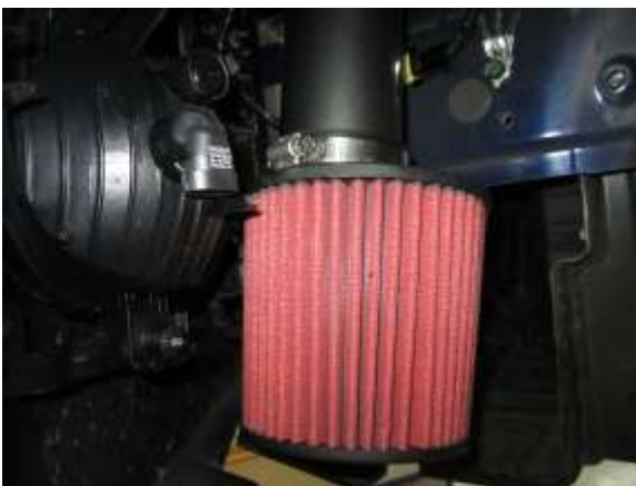
G. Inside the fender well, mount your new AEM® Dry-flow™ Air Filter (G) onto the intake tube inlet. Rotate the offset filter to clear the fog lamp and the wheel well cover, and then secure with the hose clamp.
