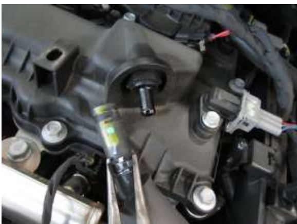
C. Disconnect PCV hose on top of the valve cover and pull it aside to expose the hose clamp at the throttle body below.
