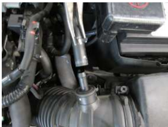
B. Disconnect the breather return hose at the stock intake tube.
