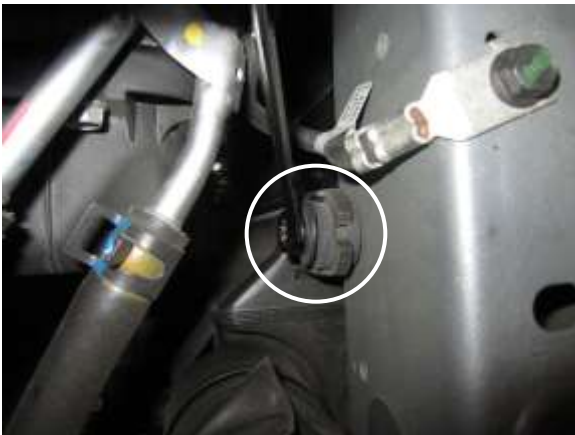
M. Under the hood, remove the 4th and final M6 bolt retaining the intake silencer to the frame support.
