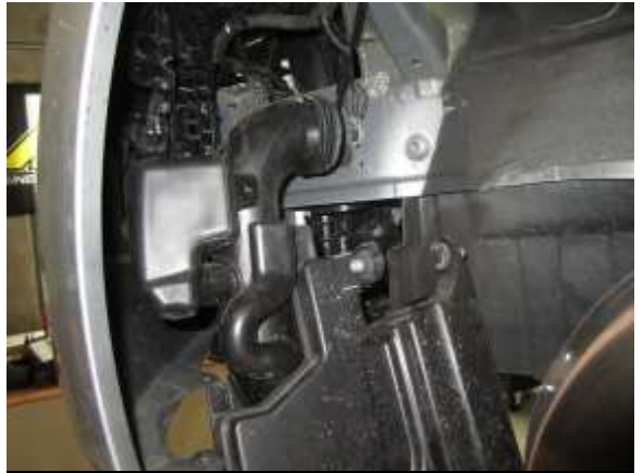
N. Lower and remove the large intake silencer from the wheel well.
