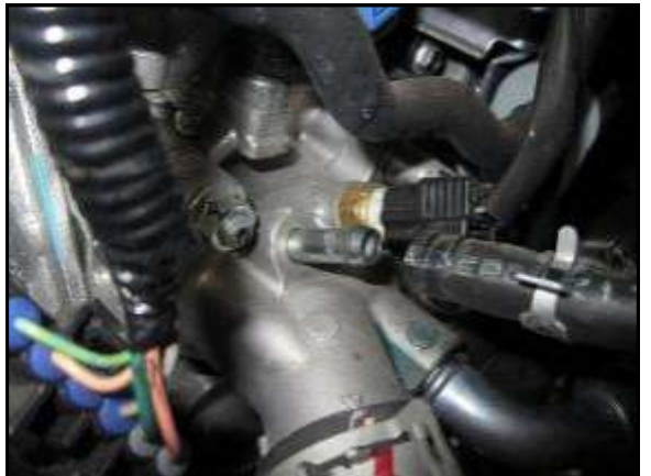
Z. Place a rag under the hose to catch any spilled coolant. Release the clip on the thermostat coolant hose and pull the hose off.
