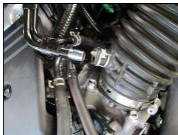
C. Release the clip on the PCV pipe and remove the pipe from the intake tube. Remove the PCV pipe from the Valve cover.
