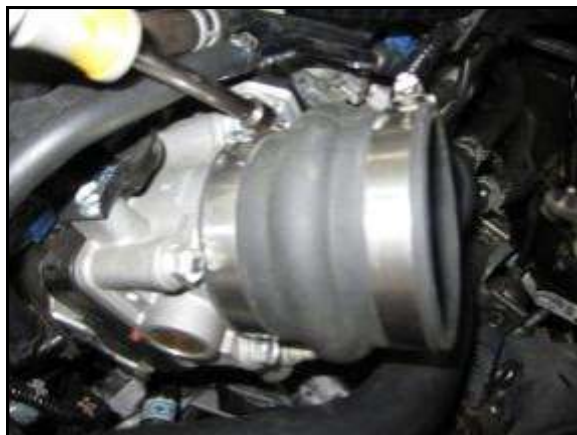
B. Install the 5-530 coupler (D) on the throttle body with the two # 48 hose clamps (E)
