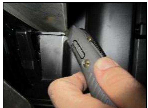
V. With a razor blade carefully cut 2" off of the plastic piece in-between the front of the bumper and radiator support for increased air flow.
