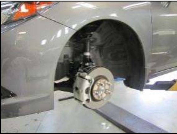
K. Remove the driver side wheel.
