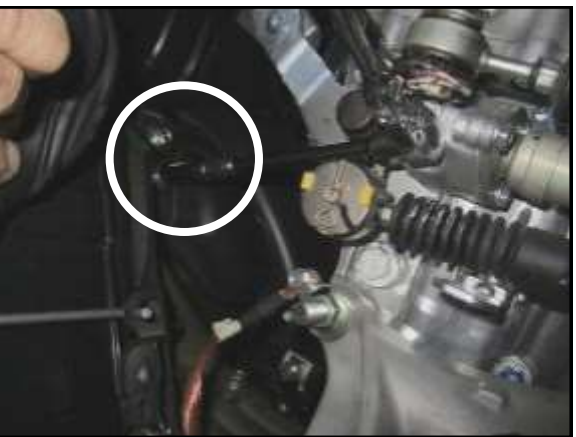
I. Remove the two M6 bolts under the battery tray for the lower intake tube.
