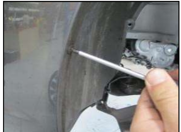
N. Remove the Philips screw.
