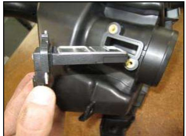
X. Remove the MAF sensor.
