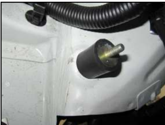
C. Install the rubber mount (J) in the OEM threaded bolt hole as shown.
