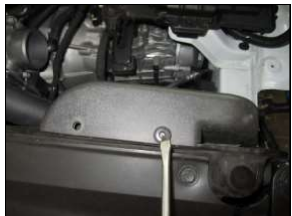
P. Push in on the center of the clips as shown and remove clips. Remove the air scoop.
