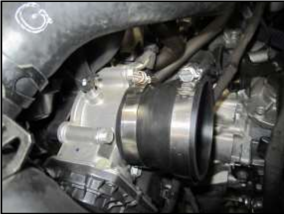
A. Install reducer coupler (B) (5-253) on the throttle body with the #40 (A) and # 48 (D) hose clamp.
