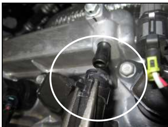
B. Release the clip on the valve cover for the PCV hose, then remove the hose from the valve cover.
