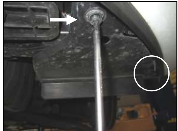
H. Remove the two lower clips on the bottom of the fender liner .
