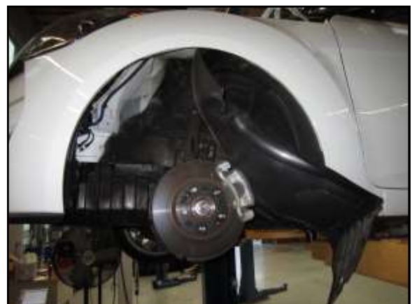
J. Move the fender liner out of the way to gain access to the resonator .
