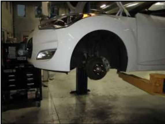
G. Raise the front of the vehicle with a jack. Support your vehicle using properly rated jack stands before wheel removal or while working under the vehicle. Remove the driver side wheel.
