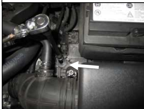
D. Loosen and remove the left 6mm bolt holding the air box.
