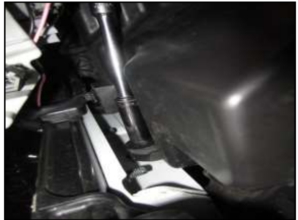
L. Remove the lower 6MM bolt on the bottom front of the resonator .
