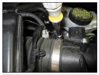
f. Lossen the hose clamp on inlet tube to the airbox.
