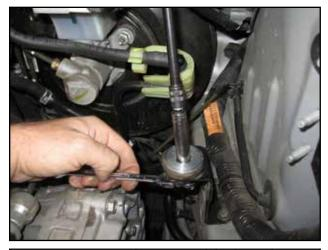
g. Once properly assembled, tighten the nuts and bolts to secure the adapter assembly.
