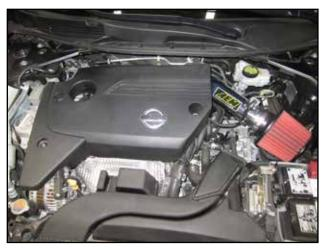
r. Make sure all the hose clamps and fasteners are tight then install the engine cover.
