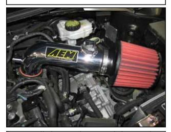
k. Install the intake pipe (1) into the throttle body coupler and align the bracket in place on rubber mount.
