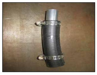
Insert nipple (8) into hose (7) and use the two (9) hose clamps on the hose as shown. Tighten the hose clamp on the nipple.
