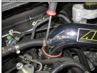
Tighten the provided (7) vent hose and (8) hose clamp to the intake tube.
