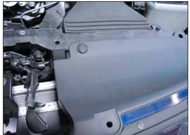
ao. Install the 8 clips to secure the radiator shroud, beginning with the clip securing the air inlet scoop in place.
