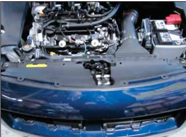
an. Reinstall the radiator shroud.
