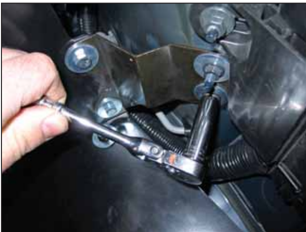
p. Once the heat shield is properly positioned, tighten all nuts to secure the heat shield in place.
