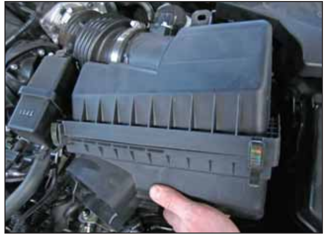
l. Lift up on the bottom of the air box to disengage but do not remove from engine bay.
