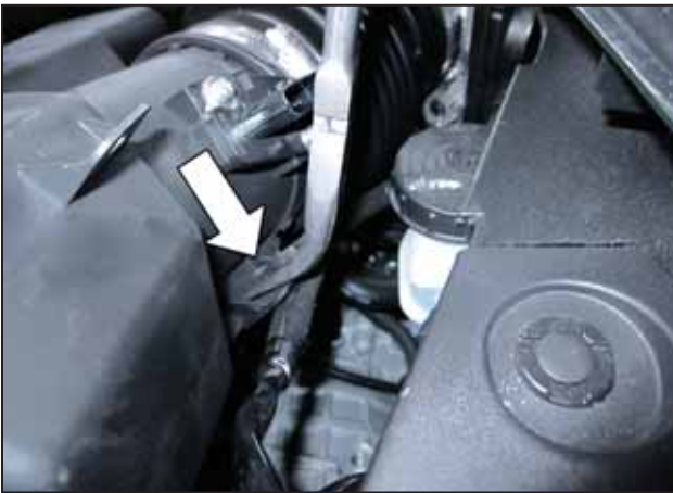
m. Remove the 2nd MAF harness clip from the back side of the air box.
