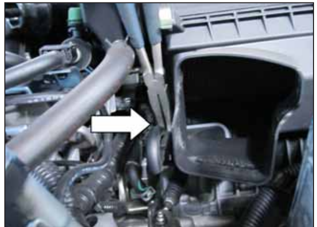
j. Remove the clip securing the transmission breather to the factory air box.
