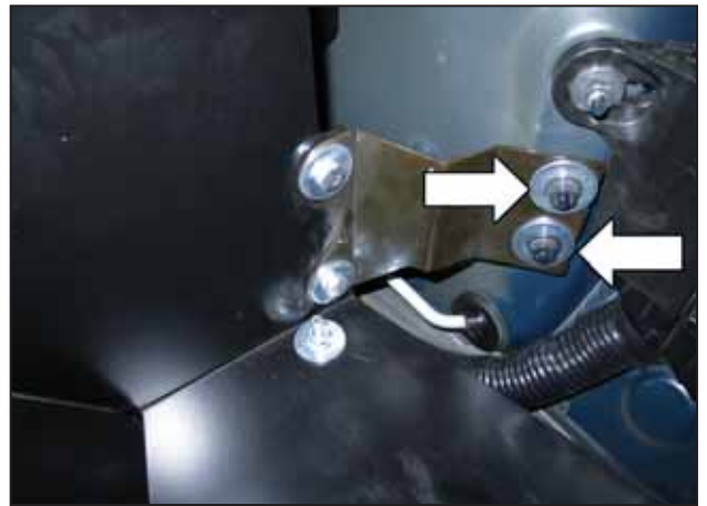
o. Align the heat shield's bracket with the two studs, secure in place using two washers (08160) and the two OEM nuts removed in step 2v.
