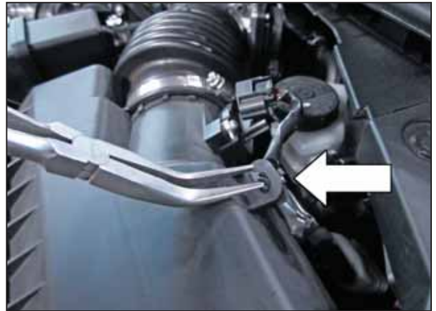
h. Release the clip securing the MAF sensor harness to the air box.
