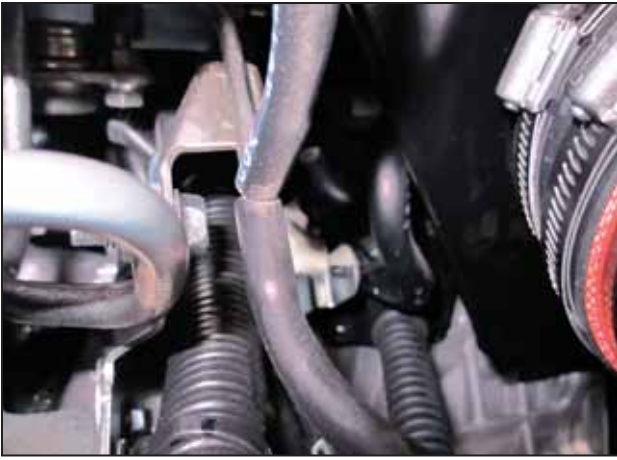
aj. Attach the transmission breather hose's clip to the heat shield from the underside.
