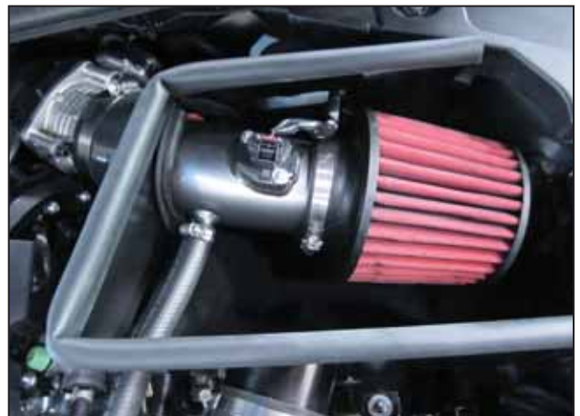
ai. Attach the PCV vent hose to the intake pipe's vent. Secure the vent hose with hose clamp (08411) and connect the MAF sensor harness plug to the MAF sensor.
