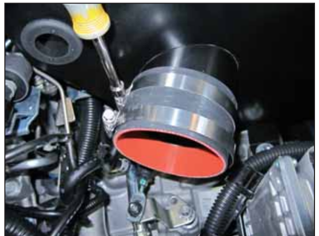
q. Install the 3.5" coupler (5-351) with two #56 hose clamps onto the heat shields inlet, tighten the hose clamp on the heat shield inlet end.
