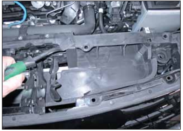
r. Remove the left clip from the lower shroud.
