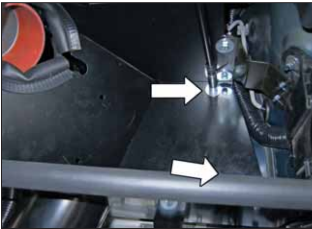
n. Secure the heat shield to the threaded bolt ends with two washers (08160) and two M6 nuts (444.460.04).
