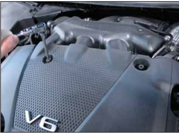
a. Remove the two 5mm Allen head bolts that secure the valve cover in place.
