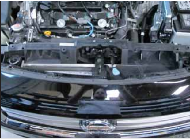
q. Remove the upper radiator shroud from the vehicle.
