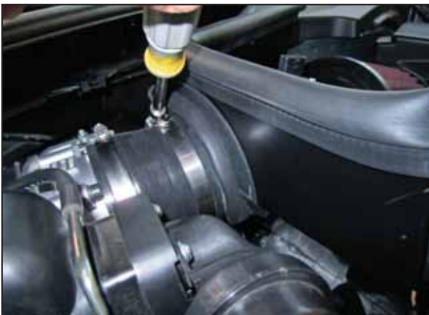
ah. Align the intake pipe with the throttle body's coupler and secure the #52 hose clamp.
