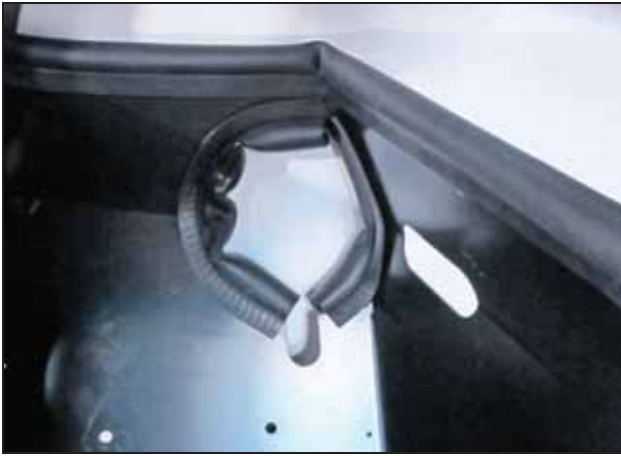
l. Install the rubber edge trim around the intake tube opening in the heat shield.
