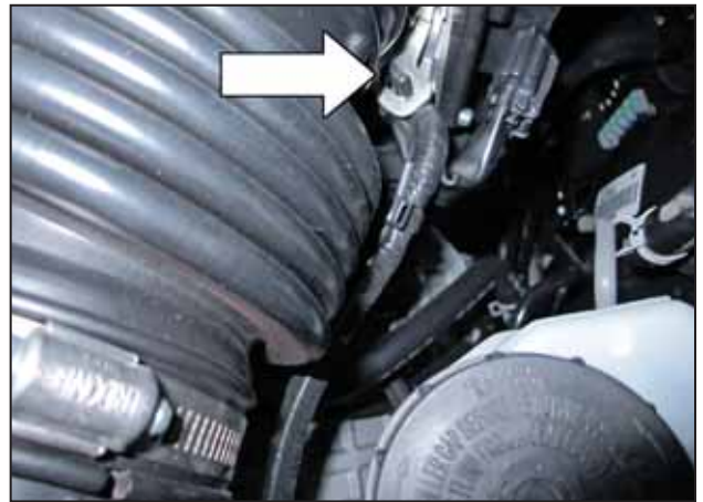
n. Remove the 3rd MAF harness clip from the inlet tube.
