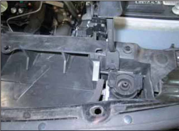
s. Remove the right clip from the lower shroud.
