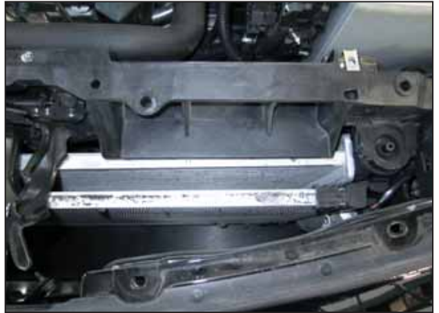
t. Remove the shroud from the vehicle.
