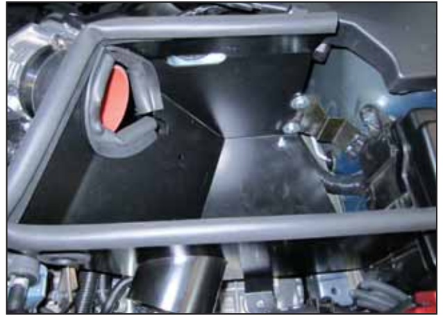
m. Place the heat shield in the vehicle's engine bay, ensuring the threaded ends of the bolts from step 3g align with the openings on the bottom side of the heat shield.
