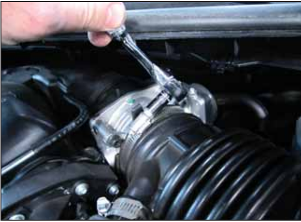
k. Loosen the hose clamp that secures the inlet tube to the throttle body.
