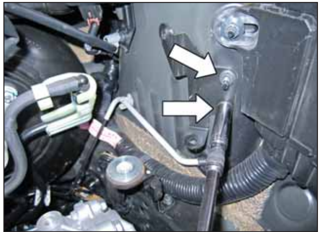
v. Remove the two 10mm bolts securing the factory air box bracket to the inner engine bay wall.
