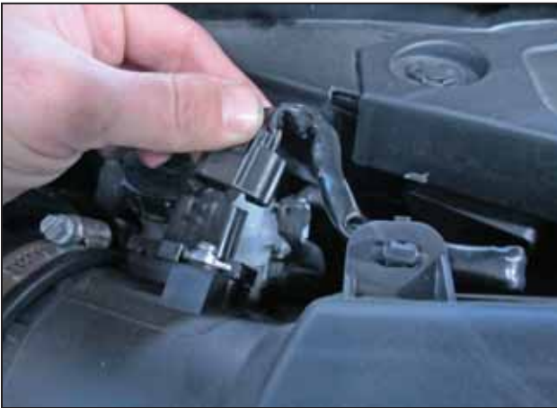
g. Unplug the MAF sensor connector.
