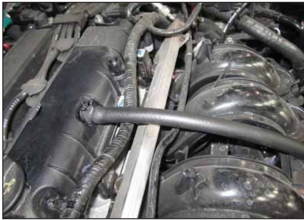
k. Using a mild soap mixture, attach the supplied 3/8 hose to the valve cover nipple and secure with the factory hose clamp.
