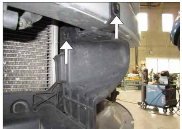
n. Loosen the two plastic clips securing the lower grill air director on the driver's side and remove. NOTE: Keeping this component on the vehicle will restrict the AEM® intake system from optimal performance.
