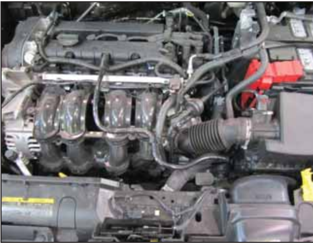
a. Stock air box system installed.
