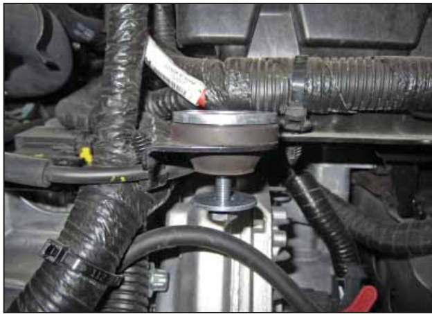
g. Slide a washer and M6 nut onto the M6 bolt as shown. Thread the bolt on about 3-4 threads.
