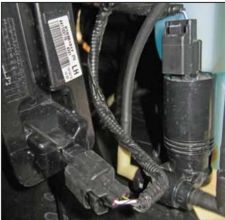
k. Pull back the front part of the wheel well plastic underlining and disconnect the front bumper light harness clips.
