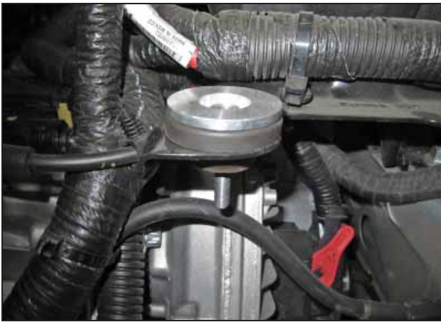
f. Insert the aluminum stand into the left rubber grommet of the factory air box mount. Slide the provided M6 bolt through the spacer and rubber grommet as shown.
