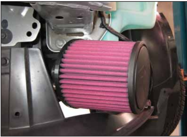
j. Install the air filter onto the lower intake pipe and secure with a #44 hose clamp. Tighten the upper and lower M6 nuts on each of the mounting brackets once adequate clearance for the air filter is achieved.
