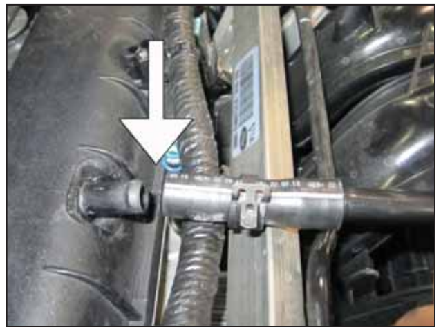
d. Using needle-nose pliers, loosen the hose clamp and disconnect the valve cover hose.
