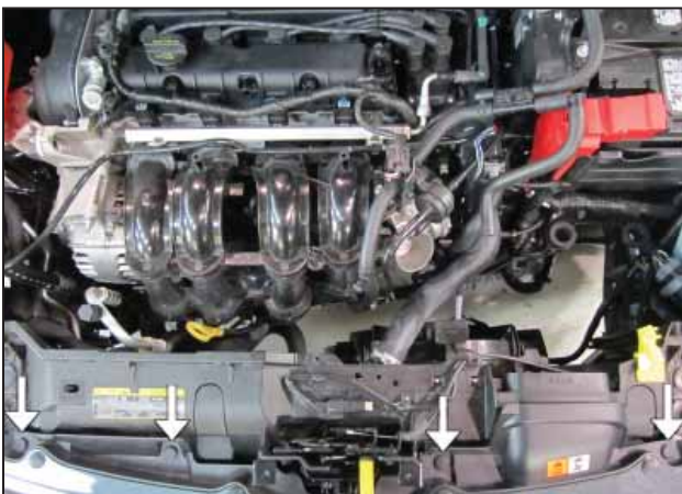
m. Remove the 4 clips above the front grill and carefully slide the bumper off.
