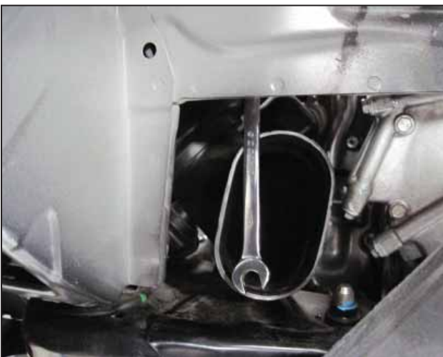
u. Loosen the two 12mm bolts on the bottom of the battery tray.
