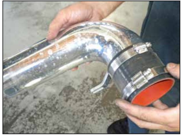
o. Install a straight coupler and two hose clamps onto the lower pipe.
