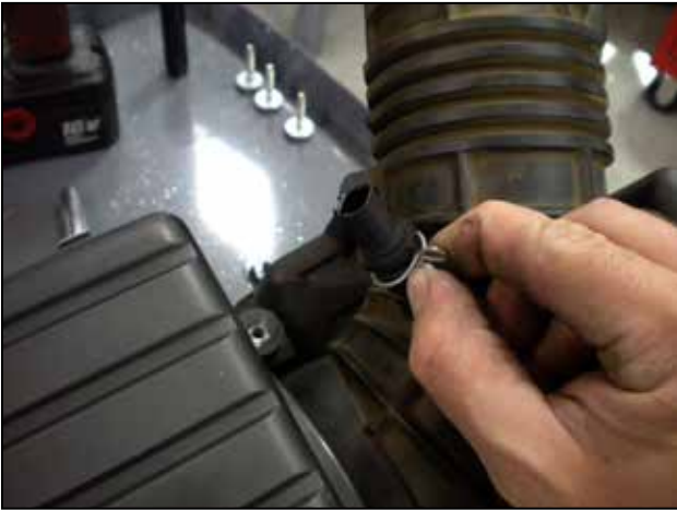
m. Remove the IAT sensor from the inlet tube.
