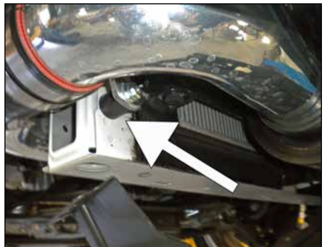
s. Secure with a washer and nut.
