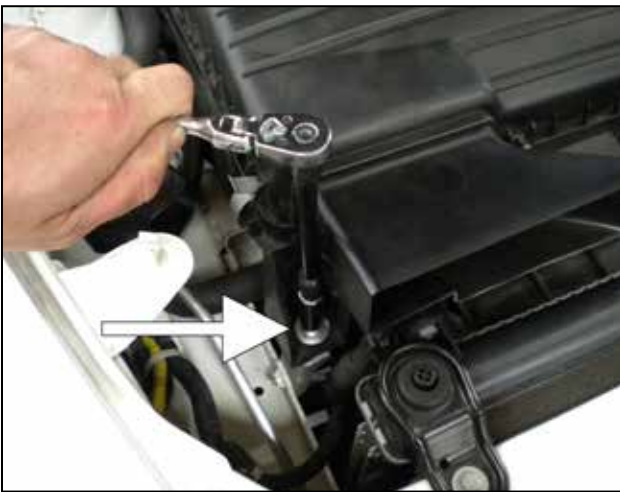
g. Remove the bolt securing the air box on the passenger side of the vehicle.
