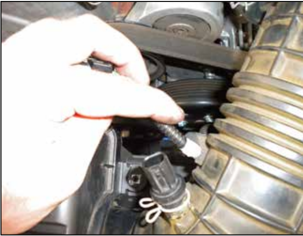
e. Disconnect the wire harness from the inlet tube.
