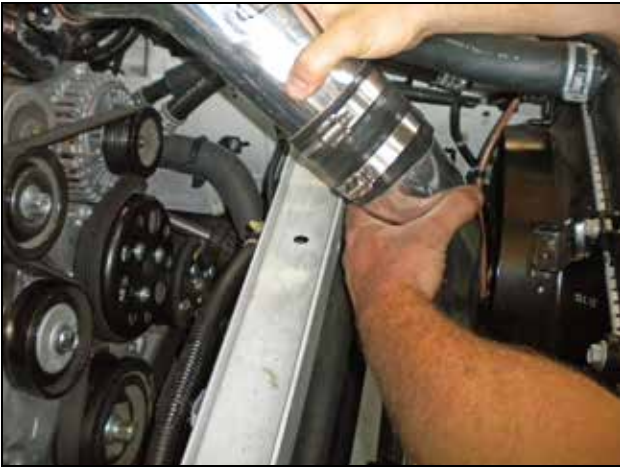
n. Connect the middle pipe to the upper pipe that is already installed.
