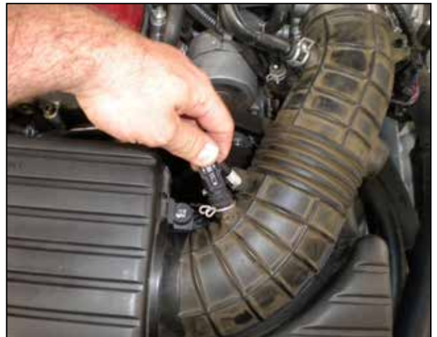
d. Disconnect the IAT sensor connector from the sensor.
