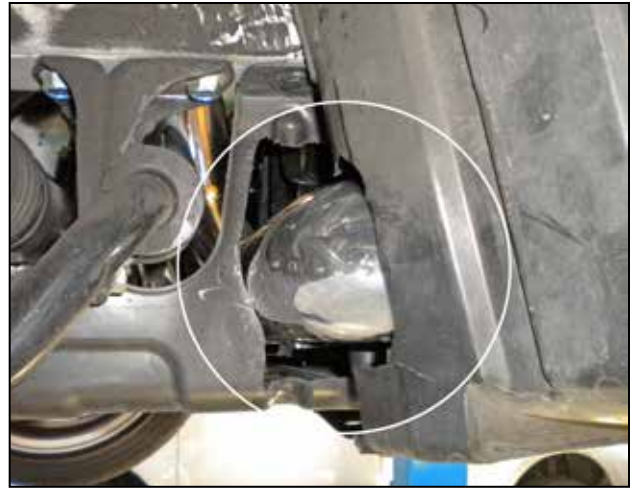
u. Reinstall the fender liner and trim to fit.
