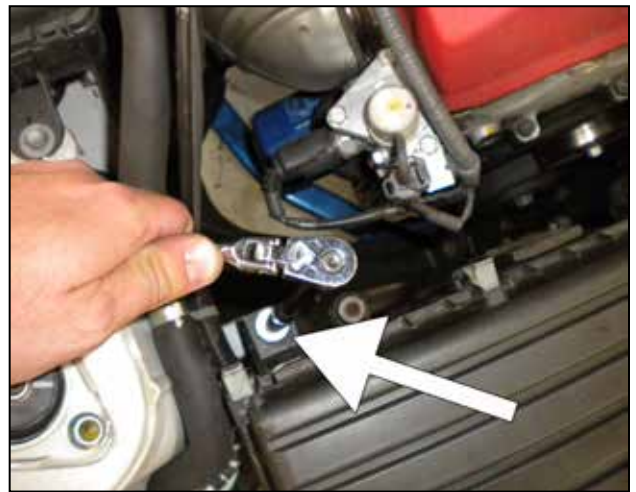
h. Remove the bolt securing the air box on the firewall side of the air box.
