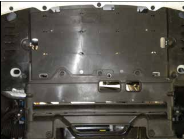
o. Remove the passenger fender liner and the bottom front and rear liner.
