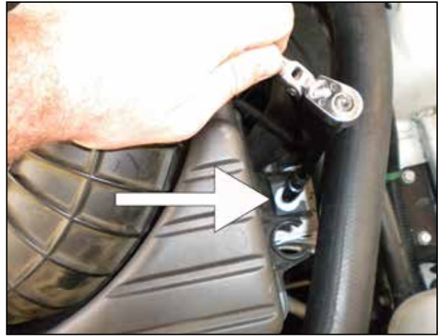
f. Remove the bolt securing the air box on the driver side of the vehicle.
