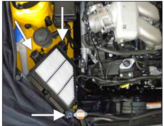
d. Unclip the MAF sensor harness from the lower half of the airbox. Remove the three M6 bolts securing the lower airbox, and remove the lower airbox.
