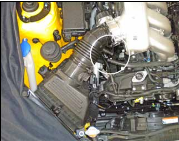
c. Unhook the crankcase vent hose by sliding back the spring clamp, then pulling the hose off of the nipple on the inlet tube. Remove the airbox lid and stock inlet tube assembly.
