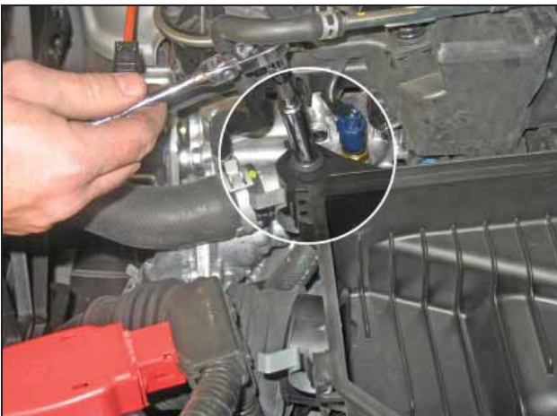
i. Remove the front bolt securing the stock air box.
