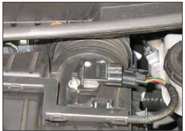
b. Disconnect the mass airflow sensor harness from the mass airflow sensor.
