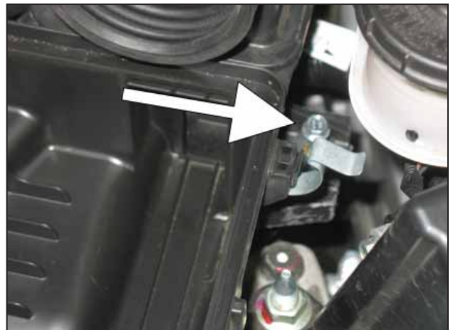
j. Remove the second bolt securing the stock air box to the vehicle.
