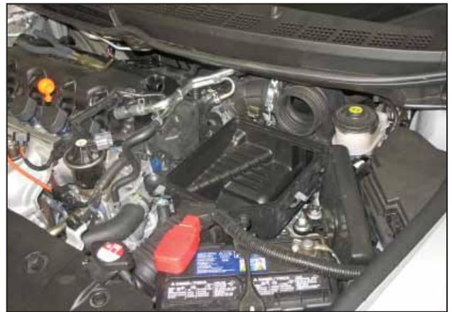
h. Remove the stock panel air filter.
