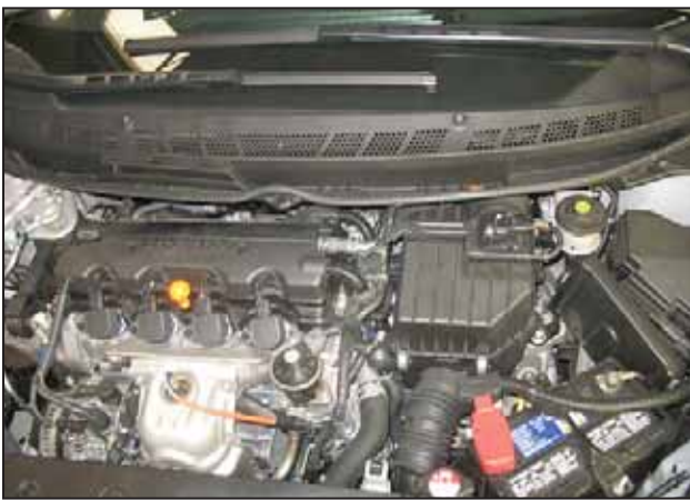
a. Stock air box system installed.
