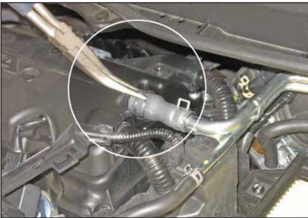
g. Disconnect the PCV hose from the valve cover.
