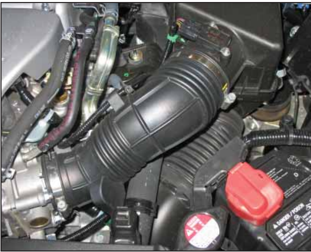
a. Stock air box system installed.
