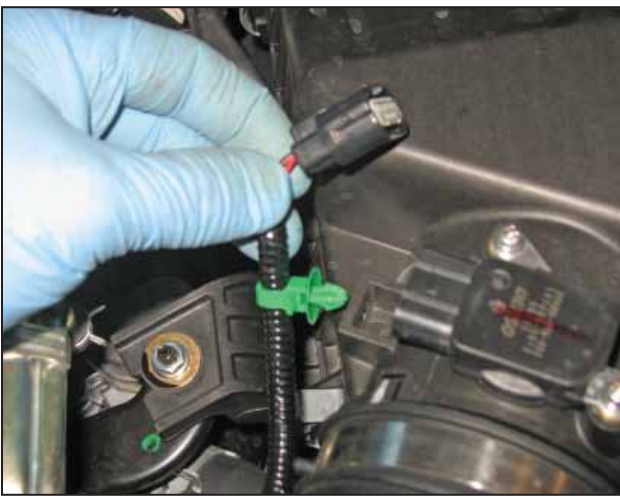
c. Disconnect the mass airflow (MAF) sensor from the vehicle.
