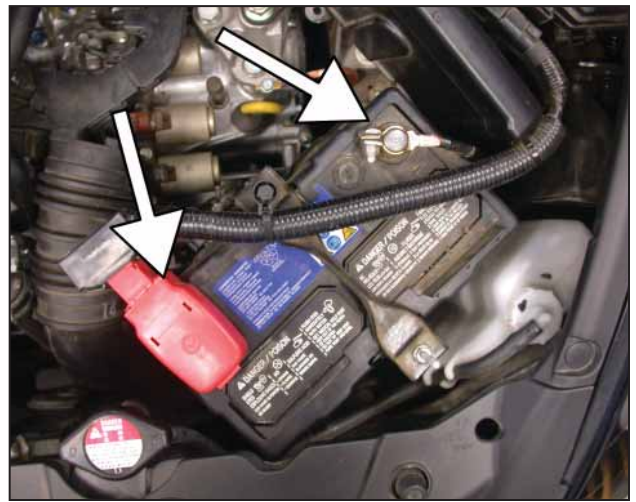
b. Disconnect the negative and positive battery terminals. Remove the battery tie down and battery according to the owner's manual.
