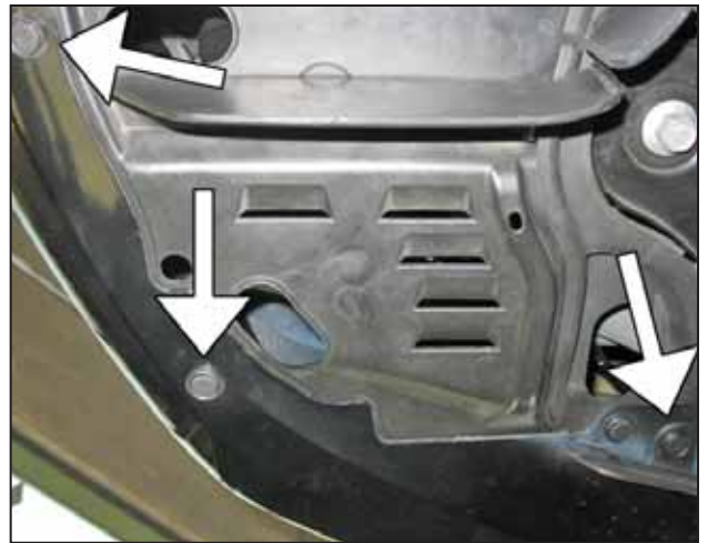
q. Remove the bottom clips holding the bottom plastic tray.
