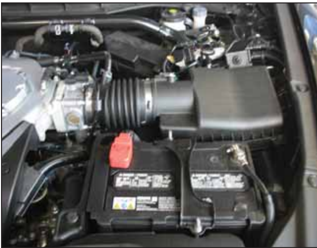
a. Stock air box system installed.
