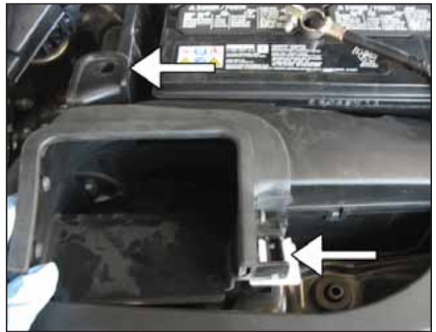
b. Remove the front inlet duct located near the battery.
