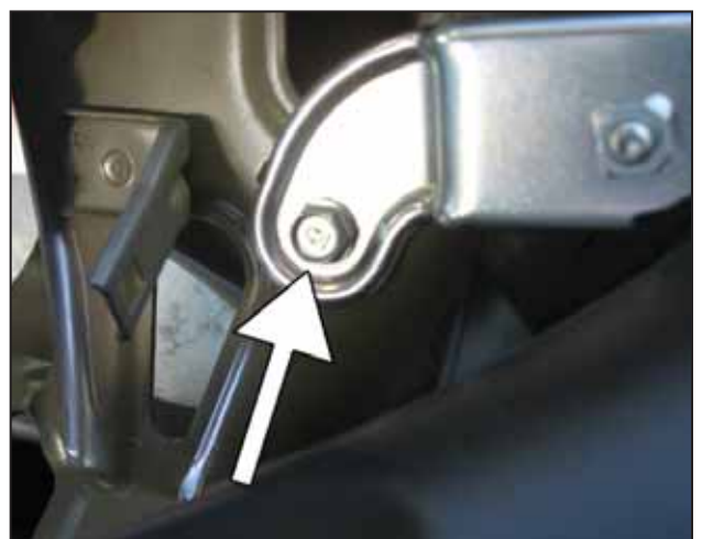
u. Underneath the battery bracket, remove the 10mm bolt that holds the air induction pipe to the battery bracket.
