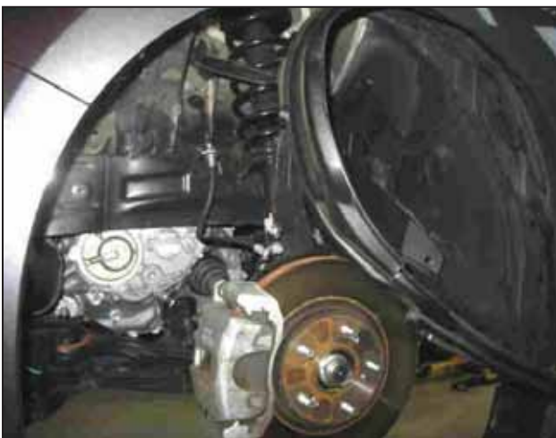
r. Push back the fender liner as shown in the picture.
