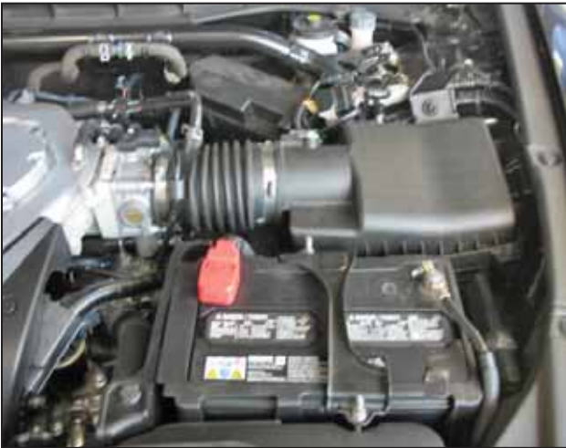
Factory air box system installed
