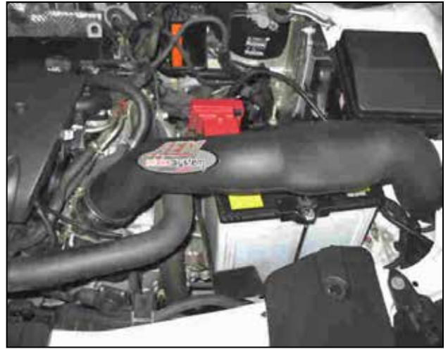
AEM® intake system installed
