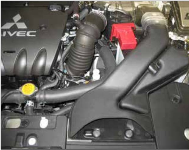
Factory airbox system installed
