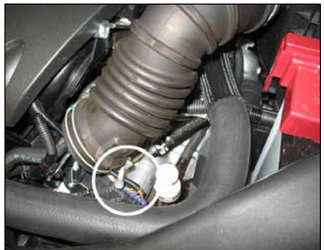
d. Using a 10mm nut driver, loosen the hose clamp on the tube on the throttle body side.
