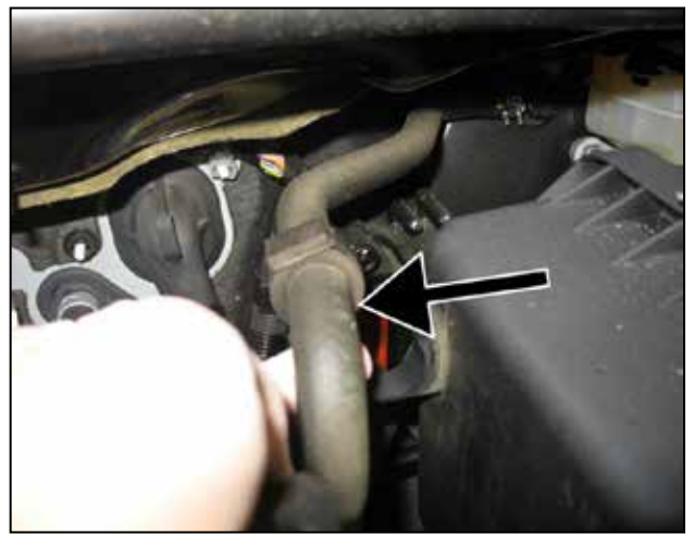
h. Remove the hose from the airbox housing near the back.
