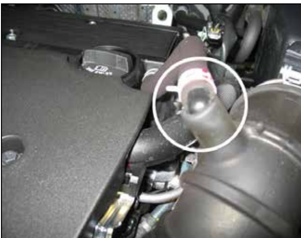
c. Remove the PCV tube from the crankcase side.
