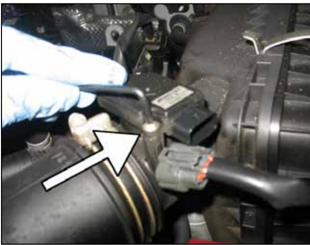
g. Remove the MAF sensor with the provided T20 L-key.
