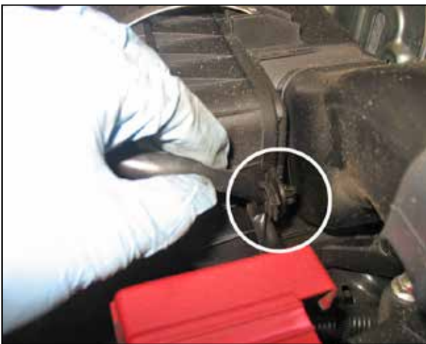
i. Remove the clip on the MAF connector wire that is attached to the airbox.
