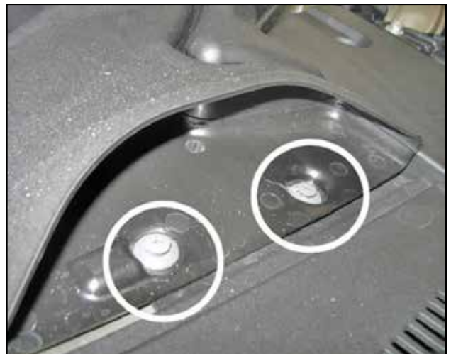
b. Remove the front section of the stock air duct, there are two Philips head screws securing it in place.
