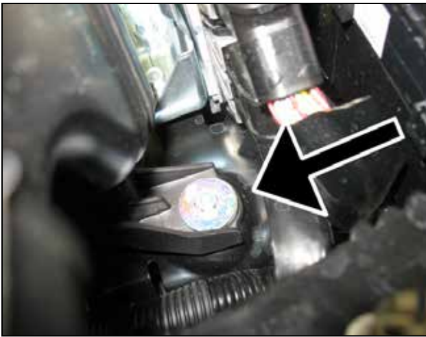
e. Remove the 10mm bolt holding the filter box to the chassis.
