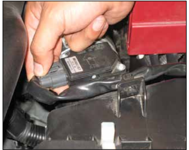
b. Disconnect the mass air flow (MAF) sensor harness connector from the MAF sensor.
