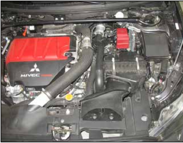
Factory air box system installed
