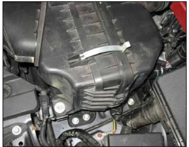
d. Remove the bolt securing the OE air box to the vehicle.
