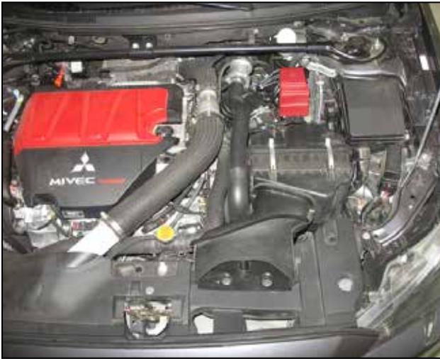
a. Stock air box system installed.
