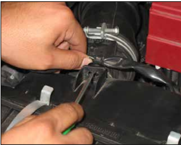
c. Using a small screwdriver remove the two tree mount zip ties from the air box housing tabs.
