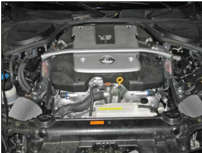
AEM® intake system installed
